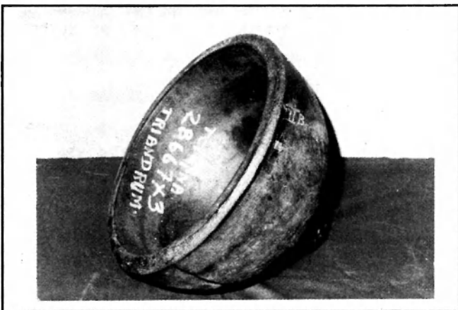
Fig. 4. Hemispherical shell forged in the Beta field
