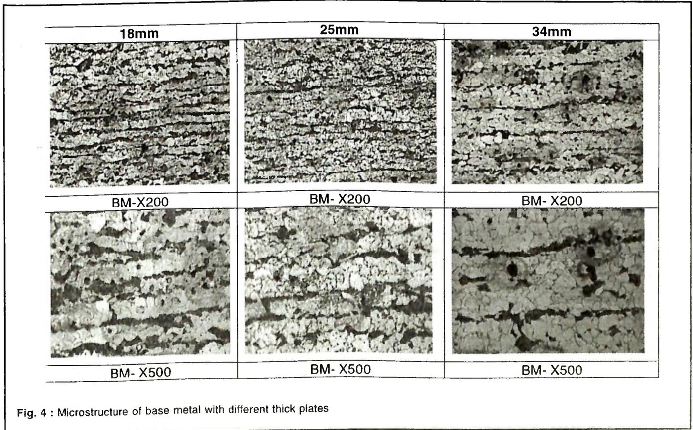
**Fig. 4 : Microstructure of base metal with different thick plates**
