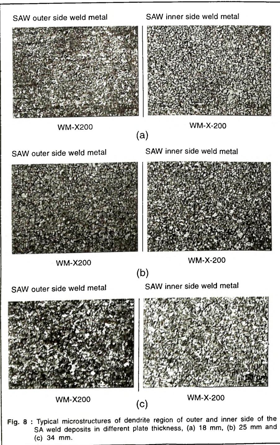
**Fig. 8 :** Typical microstructures of dendrite region of outer and inner side of the SAW weld deposits in different plate thickness, (a) 18 mm, (b) 25 mm and (c) 34 mm.
