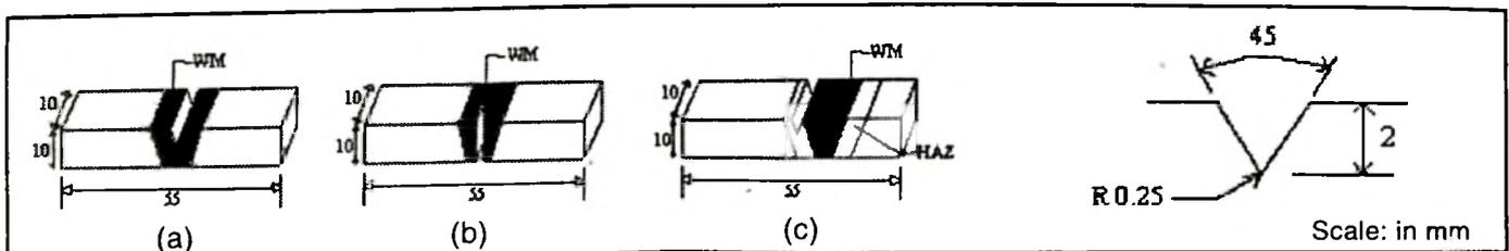
Fig. 3 : Schematic diagram of the Charpy impact specimens (a) Notch Perpendicular to weld direction (b) Notch parallel to weld direction and (c) Notch in HAZ
