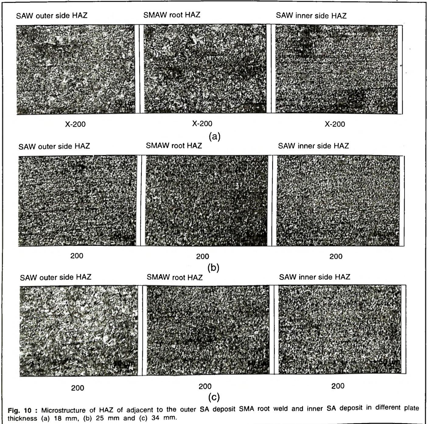
**Fig. 10 :** Microstructure of HAZ of adjacent to the outer SA deposit SMA root weld and inner SA deposit in different plate thickness (a) 18 mm, (b) 25 mm and (c) 34 mm.
