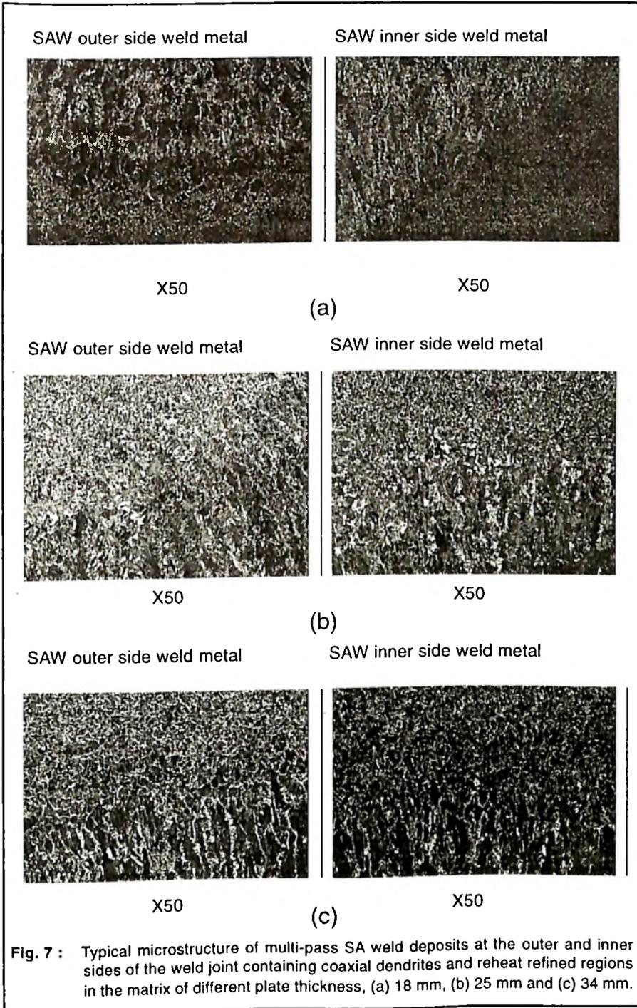
**Fig. 7 :** Typical microstructure of multi-pass SA weld deposits at the outer and inner sides of the weld joint containing coaxial dendrites and reheat refined regions in the matrix of different plate thickness, (a) 18 mm, (b) 25 mm and (c) 34 mm.
