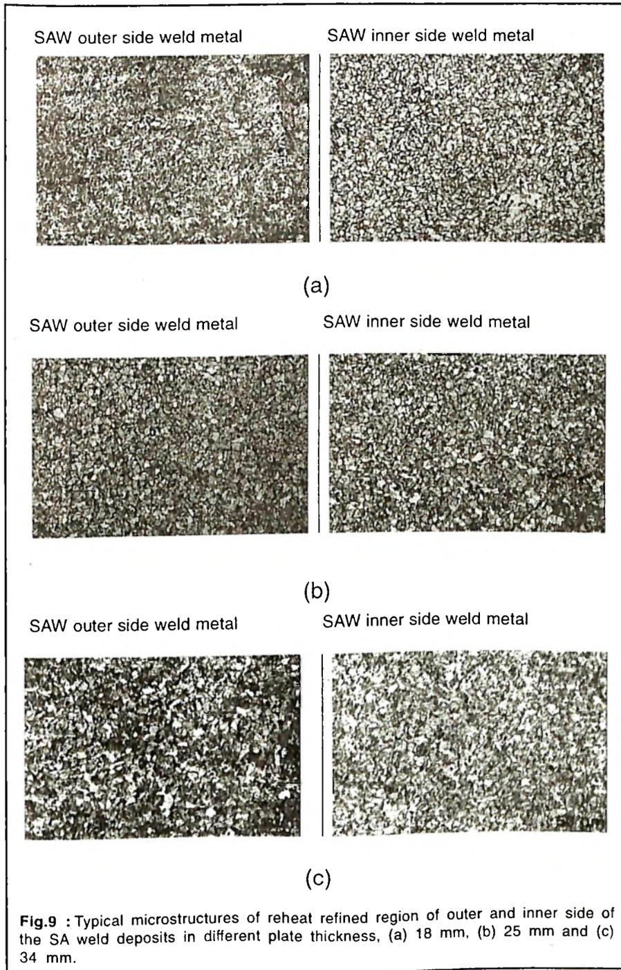
**Fig.9** : Typical microstructures of reheat refined region of outer and inner side of the SA weld deposits in different plate thickness, (a) 18 mm, (b) 25 mm and (c) 34 mm.
