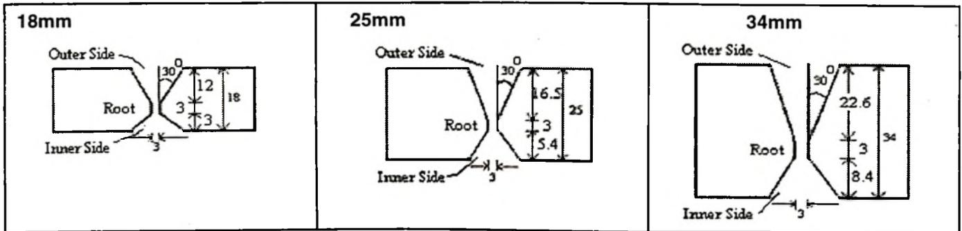
Fig. 1 : Schematic diagram of the weld grooves in reference to the fabrication of penstock liners of different plate thickness.
