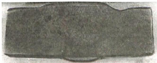
Fig-1 Macro view of the weld-joint.
