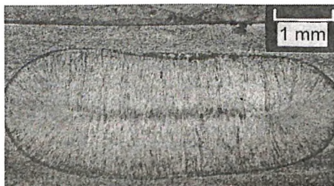
Figure 1. Typical weld nugget in austenitic stainless steel.
