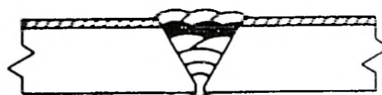
Complete Welding from Clad Side
