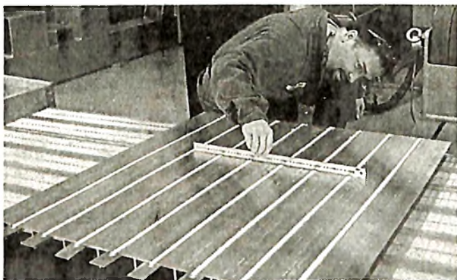
Figure : 1. Friction stir welded, straight panels under inspection at ESAB FSW Center of Excellence in Sweden
