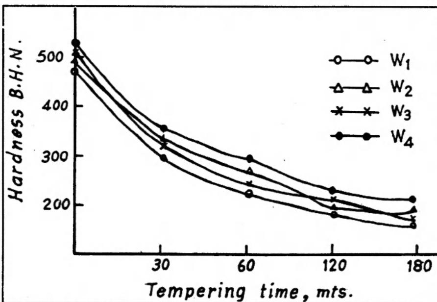
Fig 1. Hardness versus Tempering time plot for different S.G. Iron Weld metal
