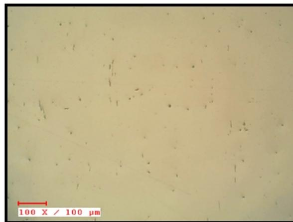
**Fig. 3 : Inclusion in the 90 mm thick plate**
