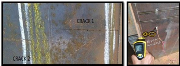
Fig. 5 : The longitudinal crack on the surface
