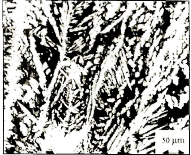
Fig. 2 : Microstructure of SMAW weld metal showing the morphological features of austenite
