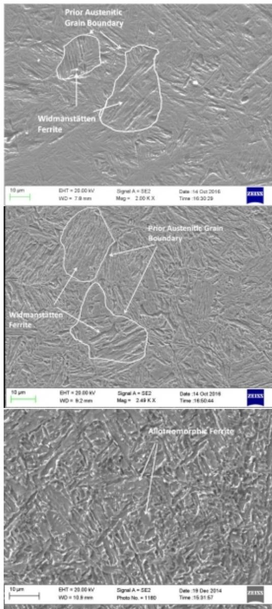
**Fig. 3 : SEM microstructure of FSW and MMAW welded nugget/stir zone of (a) 24 mm steel, (b) 8 mm steel and (c) 24 mm steel showing prior austenite grain boundary, widmanstätten ferrite and allotriomorphic ferrite.**
