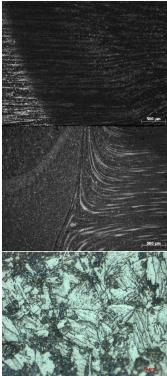
**Fig. 5 : Optical microstructure of FSW welded TMAZ zone of (a) 8 mm steel, (b) overlap stir zone in 24 mm steel and (c) at 2500X.**
