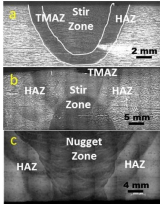
**Fig. 2 : Mosaic macrostructure of welded steel (a) 8 mm-FSW, (b) 24 mm-FSW and (c) 24 mm-MMAW.**
