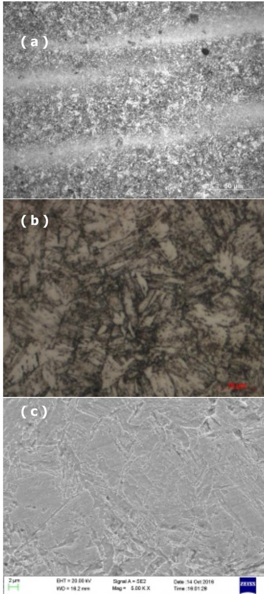
**Fig. 1 : Optical and SEM microstructure of quenched and tempered HSLA steel at magnification of (a) 500X, (b) 2500X and (c) 3000X showing banded ferritic structure with iron carbide.**
