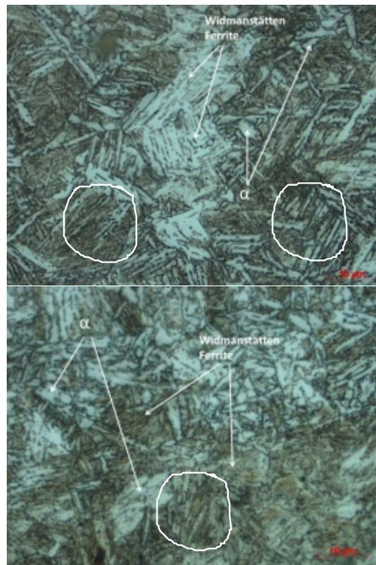
**Fig. 4 : Optical microstructure of FSW welded nugget/stir zone of (a) 8 mm steel and (b) overlap stir zone in 24 mm steel showing widmanstätten ferrite, α-ferrite and martensite.**
