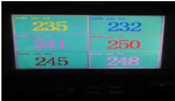
Fig. 11: Calibrated temperature reading indicates good temperature profile through reading of six thermocouples. Top row indicates temperature of inner side of pipe of depth 50mm
