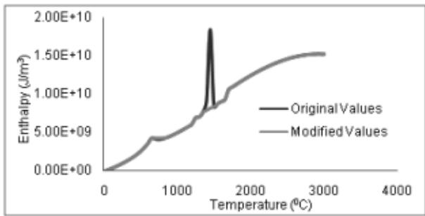
**Fig. 7 : Variation of calculated and modified values of enthalpy of AISI 430.**
