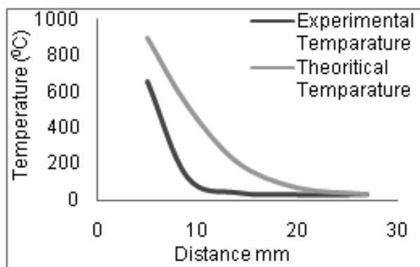
**Fig. 18 : Temperature distribution curves at 25 s**
