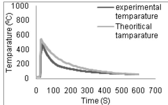
**Fig. 13 : Experimental and theoretical cooling curves at point 'b'.**
