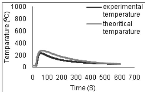
**Fig. 15 : Experimental and theoretical cooling curves at point 'd'.**
