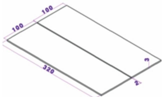
**Fig. 1 : Butt weld setup of FSS plate.**
