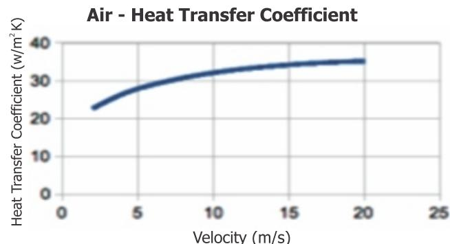
**Fig. 8 : Air heat transfer coefficient with velocity [7].**
