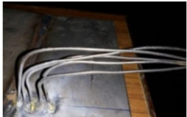
**Fig. 4 : Plate after welding with thermocouple**
