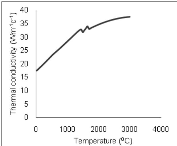
**Fig. 6 : Variation of thermal conductivity of AISI 430 with temperature.**
