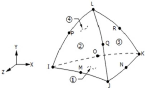
**Fig. 9 : 10-Node Tetrahedral thermal solid (SOLID87)**
