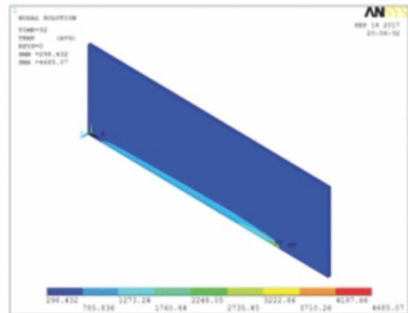
**Fig. 22 : Temperature contour plot on plate at 32 s**
