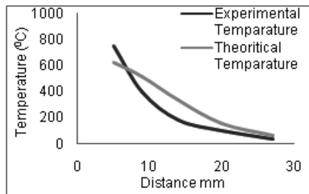
**Fig. 19 : Temperature distribution curves at 32 s**
