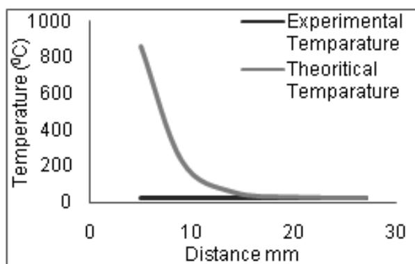
**Fig. 17 : Temperature distribution curves at 21 s**
