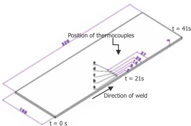
**Fig. 2 : Geometry of plate with position of thermocouples.**
