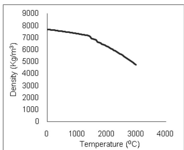
**Fig. 5 : Variation of density of AISI 430 with temperature.**
