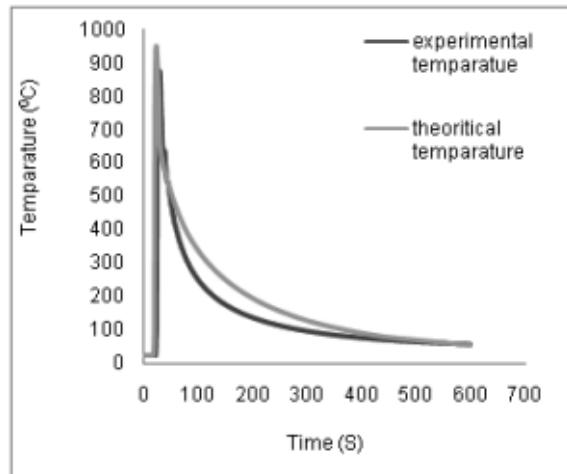
**Fig. 12 : Experimental and theoretical cooling curves at point 'a'.**
