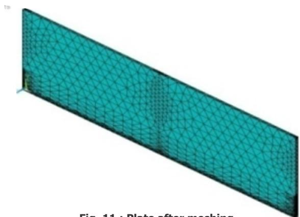
**Fig. 11 : Plate after meshing**
