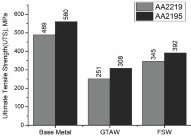
Fig. 3 : Ultimate tensile strength of BM, GTAW and FSW of 2219 & 2195 alloy
