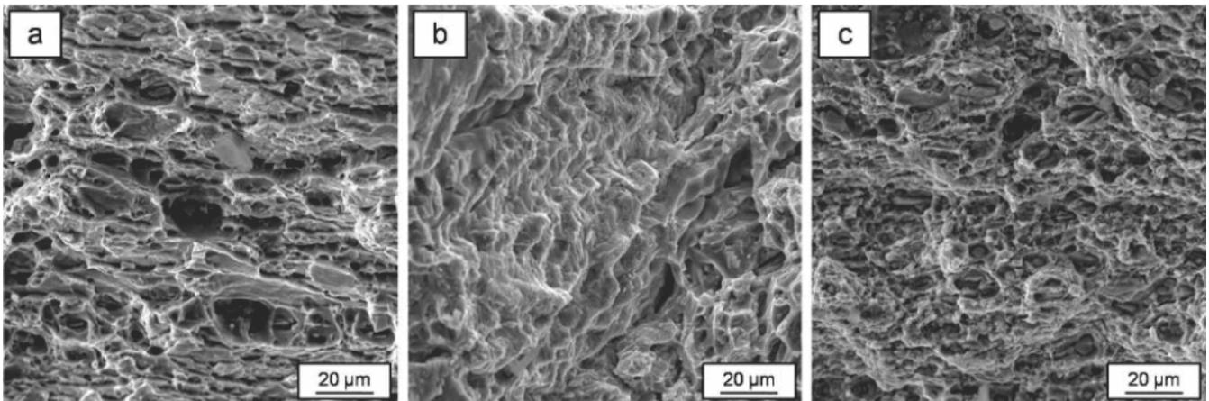
Fig. 6 : Fractographs of a) BM, b) GTAW and c) FSW of 2195 alloy
