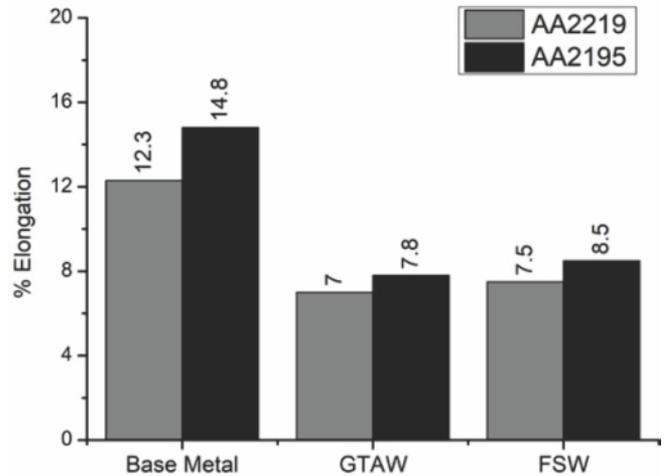
Fig. 5 : % Elongation of BM, GTAW and FSW of 2219 & 2195 alloy
