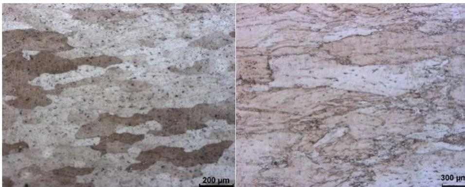
**Fig. 1 : Base material microstructure of a : 2219 and 2195 alloy**
