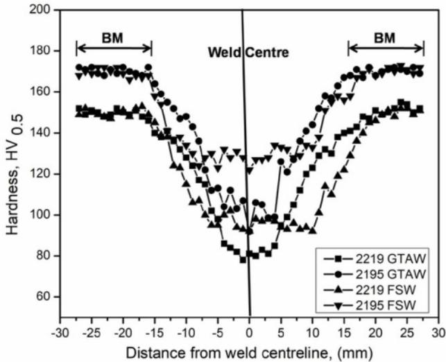
**Fig. 7 : Microhardness survey across the 2219 and 2195, GTAW and FSW welds**
