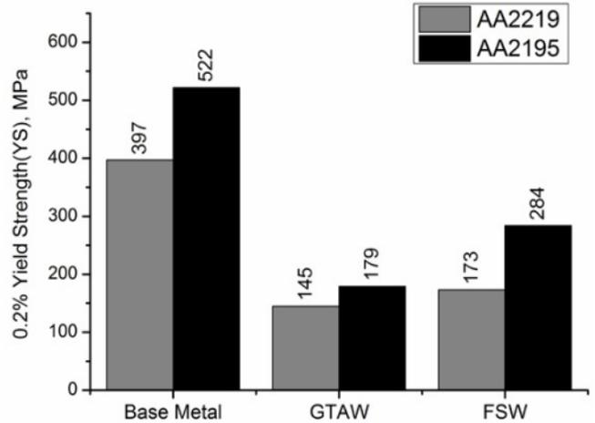
Fig. 4 : Yield strength of BM, GTAW and FSW of 2219 & 2195 alloy
