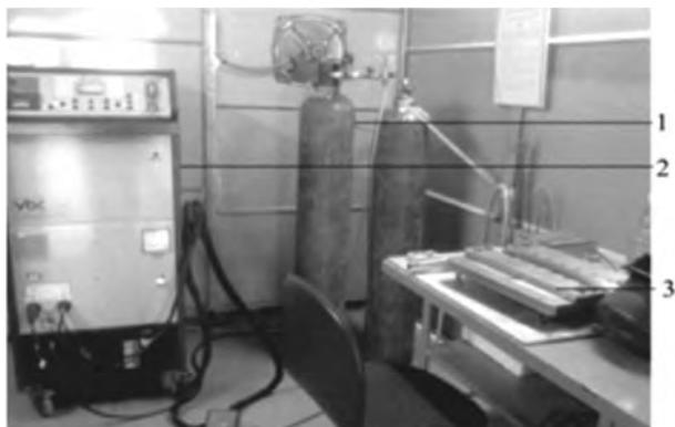
**Fig. 2 : Experimental setup - (1) Argon Gas cylinder (2) IPTIG Welding Machine (3) Welding Fixture**
