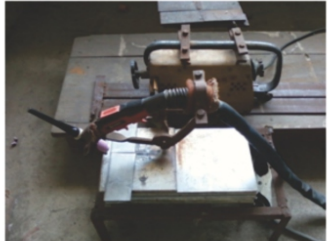
Fig.2 : Experimental set-up for butt joining of plates
