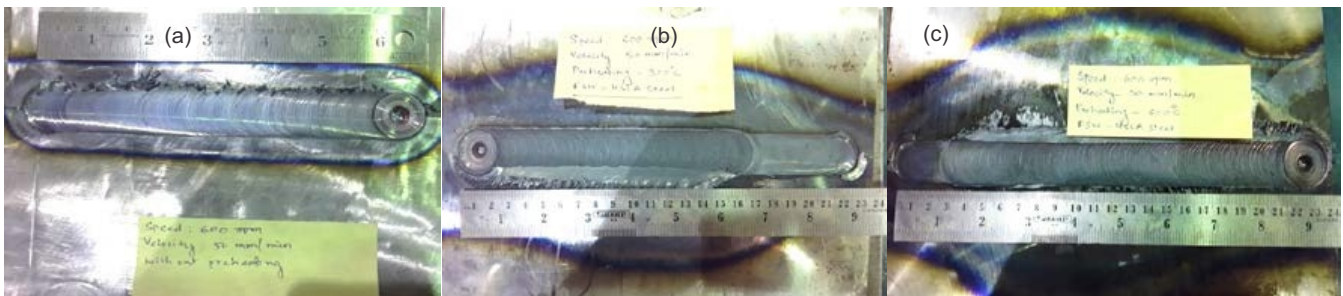
Fig. 2 : Photographs showing FSW welded plates carried out at (a) room temperature, (b) 300 °C and (c) 600 °C respectively.
