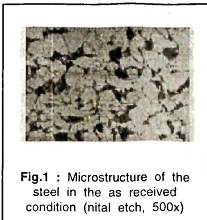
**Fig.1 :** Microstructure of the steel in the as received condition (nital etch, 500x)
