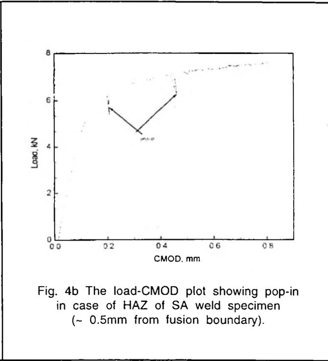
attributed this apparent increase in the fracture toughness to ductile tearing between the crack tip and the HAZ close to the fusion boundary, forcing the crack to deviate into the softer microstructural regions such as FGHAZ or the weld metal. Thus, the crack tip experiences a mixed mode of opening (tensile) and shear loading enhancing the apparent load bearing capacity of the
