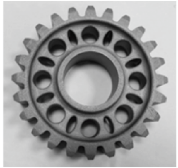
Fig. 11 : Spur gear produced by additive manufacturing after topology optimization
