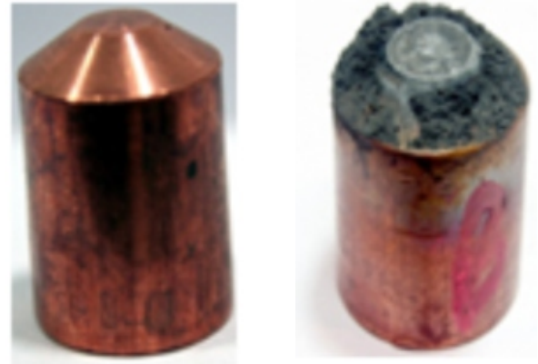
Fig. 9 : RSW: New and used Cu-Cr-Zrtruncated cone electrode capswith 6mm face diameter (for GA steel)
