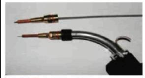
Contact tip size, liner size and wire diameter Ensure that the contact tip is the correct size and fits tightly. Ensure the gas nozzle is free from spatter.
