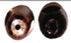
Contact tips and gas nozzle Remove spatter and replace
