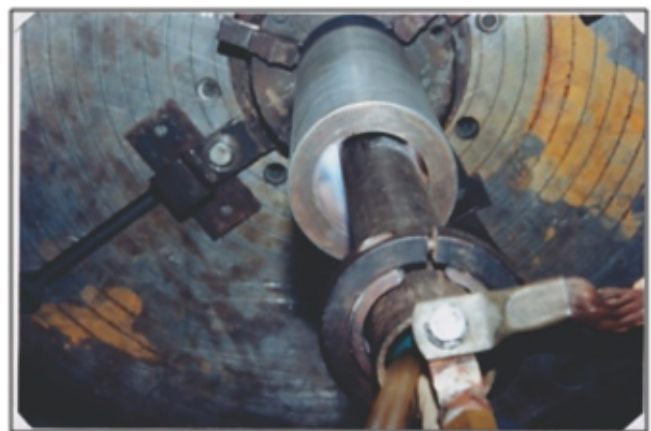
Fig. 9 : (a) Hardness profiles for Colmonoy hardface deposits made by TIG (GTA) and PTAW processes; and (b) Hardfacing of grid plate sleeve (inner diameter ~80 mm) using indigenously designed PTAW torch.
