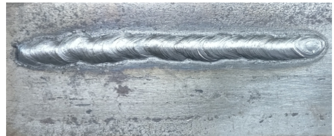
Fig. 9 : Spatterless welding joint made using 3.15mm E6013 electrode at current 120A
