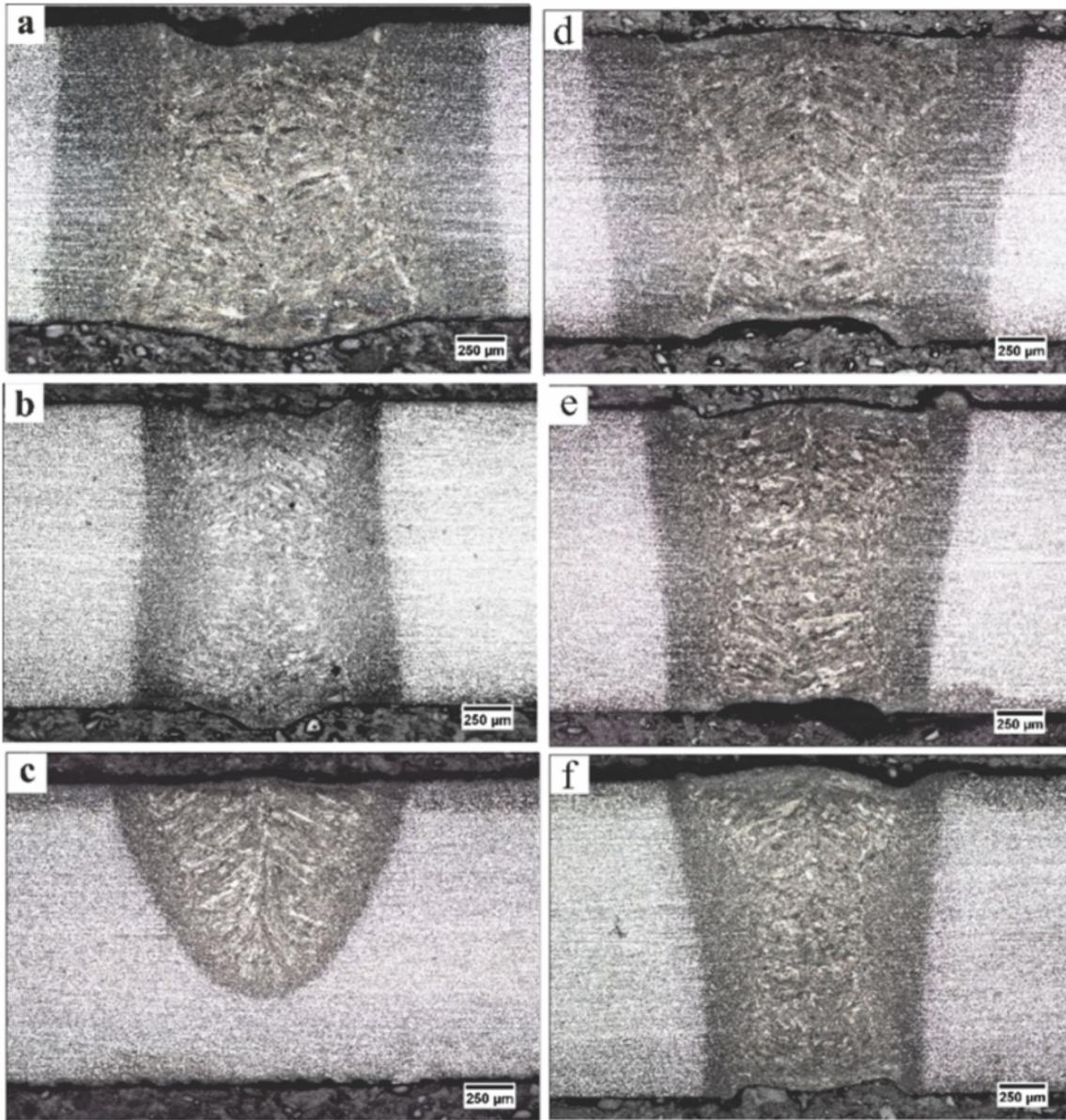
**Fig. 1 : Micrographs of weld structures of 2500 W and 3500 W**
