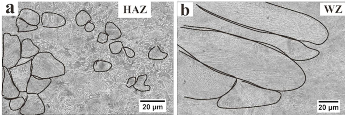
Fig. 6 : SEM Images of HAZ and WZ BW-252 [(a) HAZ, (b) WZ]
