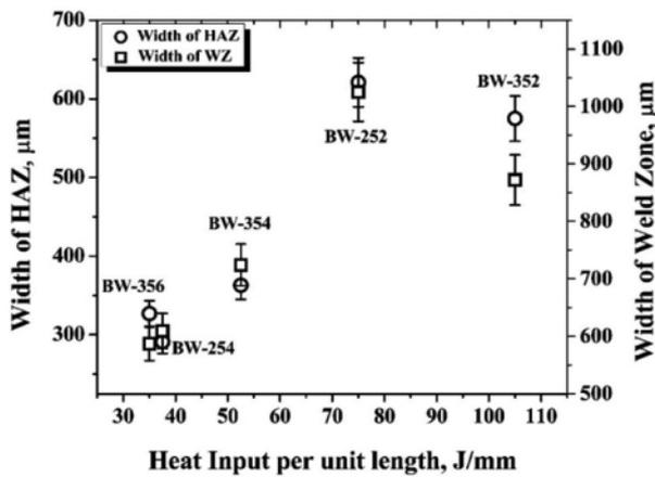
**Fig. 2 : Variation of average widths of HAZ and WZ with Heat Input**
