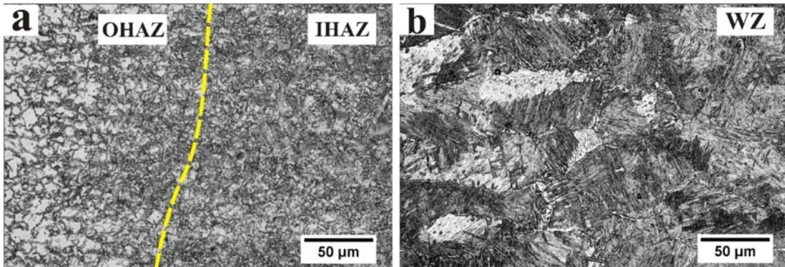
**Fig. 5 : Optical Microstructure of HAZ of BW-252 showing Inner HAZ, outer HAZ and Weld Zone**
