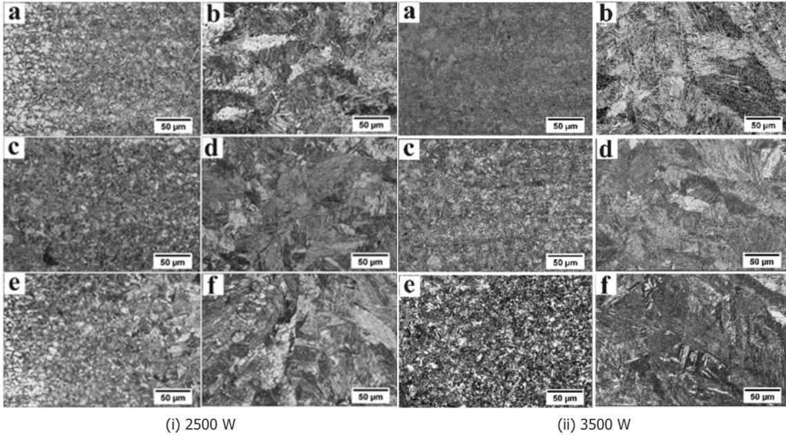
**Fig. 4 : Microstructure of HAZ and Weld Zone of Beam Power**
