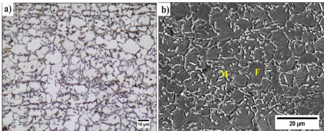
**Fig. 3 : Base material microstructure of DP 600 (a) Optical Micrograph (b) SEM micrograph**
