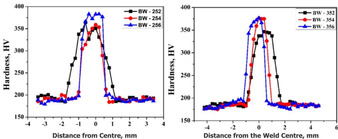
Fig. 7 : Microhardness of Bead on Plate welded structures [(a) Hardness profile of 2500 Beam Power, (b) Hardness Profile of 3500 W beam Power]
