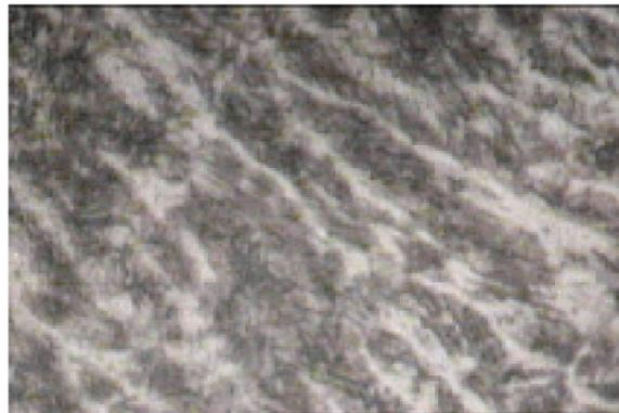
(e) V= 26 V, I= 130 A, S= 414 mm/min, Q= 0.392 kJ/mm, experiment No. 5
