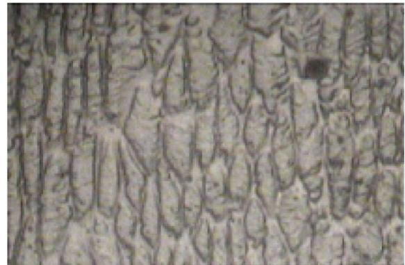
(f) At V= 28 V, I= 145 A, S= 472.8 mm/min, Q= 0.412 kJ/mm, experiment No. 6
