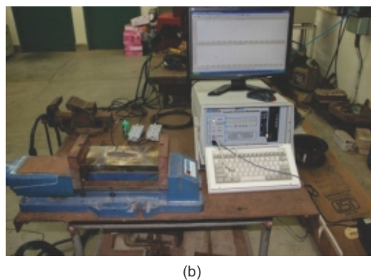
Fig. 1: (a) G-BOP sample and (b) test set up for AE data acquisition during G-BOP test
