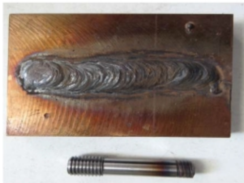
Fig. 10 : (a) Photograph of Implant test sample failed at 1800 kg load (b) AE signal for the sample
