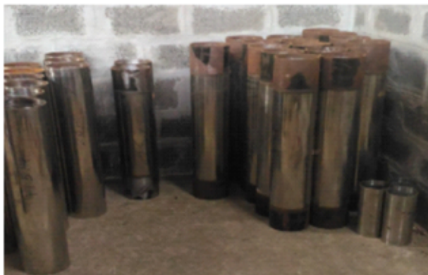
Fig. 2 : Manually Welded pump motor body
