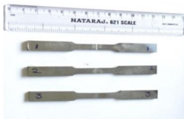
Fig. 2 : Tensile samples from laser welds
