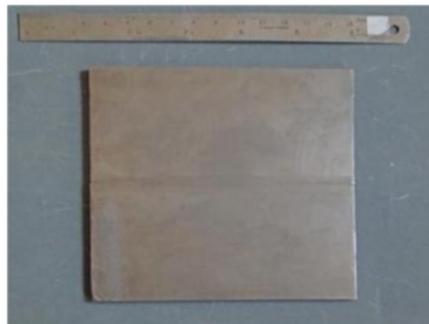
Fig. 1 : Plate –to–plate laser welded bainitic steel
