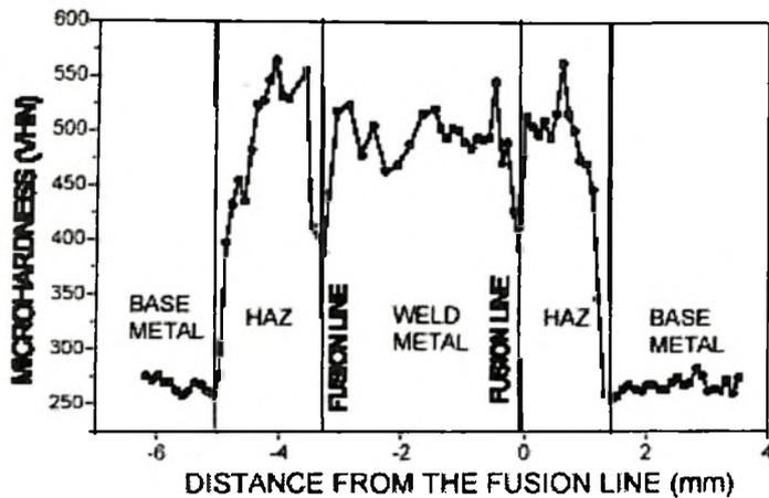
Fig. 8 Hardness profile across the weld for the UT-HST Specimen
