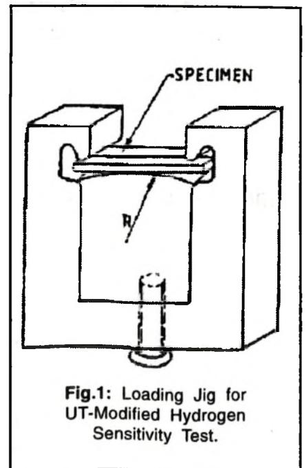
**Fig.1: Loading Jig for UT-Modified Hydrogen Sensitivity Test.**
