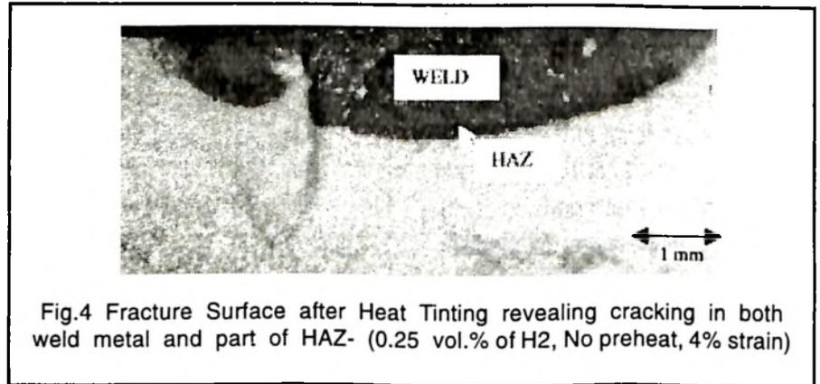
Fig.4 Fracture Surface after Heat Tinting revealing cracking in both weld metal and part of HAZ- (0.25 vol.% of H<sub>2</sub>, No preheat, 4% strain)
