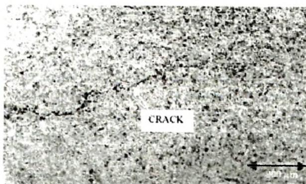
Fig. 6 Microstructure near the crack tip at HAZ showing propagation of crack along prior austenite boundaries
