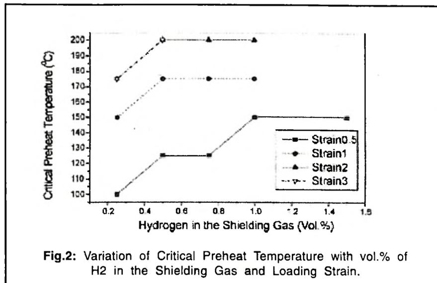
Fig.2: Variation of Critical Preheat Temperature with vol.% of H2 in the Shielding Gas and Loading Strain.
