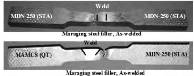
MDN-250 : Maraging Steel; MAMCS : Medium Alloy Medium Carbon Steel; STA : Solutionised and aged; QT : Quenched and tempered
