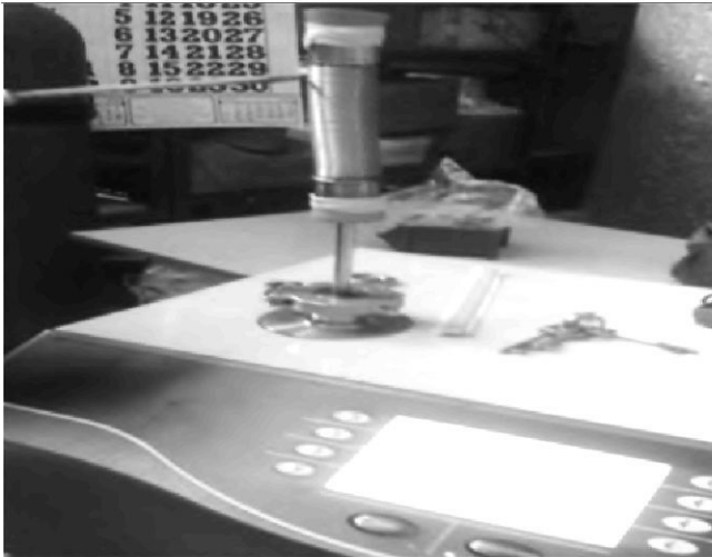
Fig. 9 : Helium leak test of cryogenic bellows
