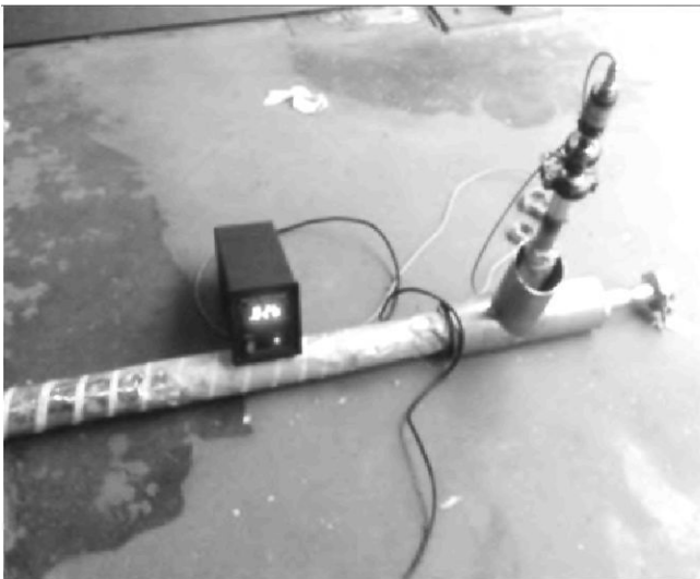
Fig. 10 : Vacuum and helium leak test of LN 2 transfer line
