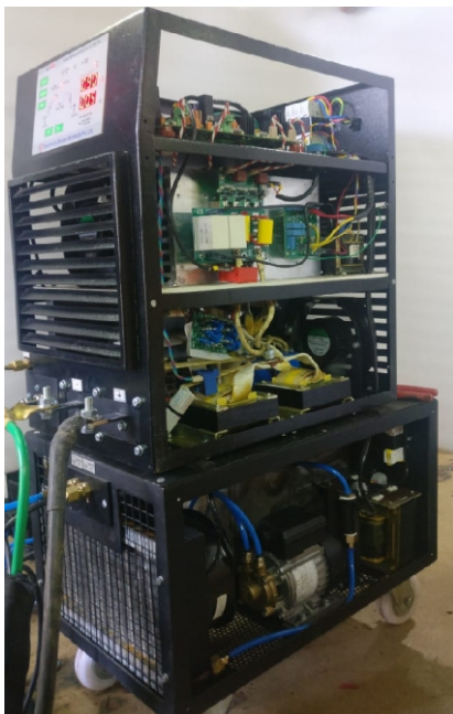
Fig. 4 : Water-cooled 300A power controller for multi-functional TIG welding applications
