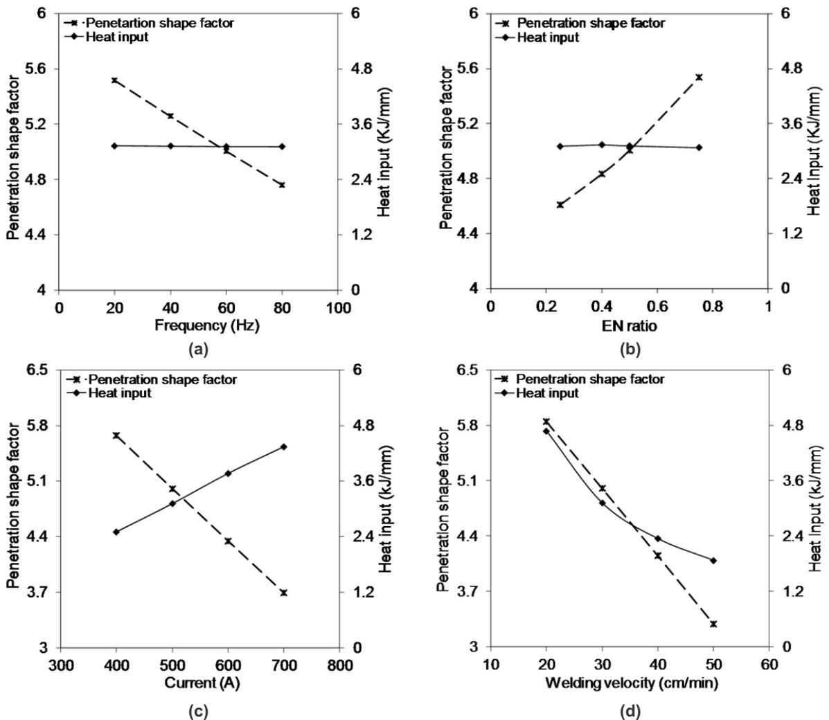
**Fig. 4 :** Effect of (a) Frequency at E=0.5, I= 500 A and V=30 cm/min
