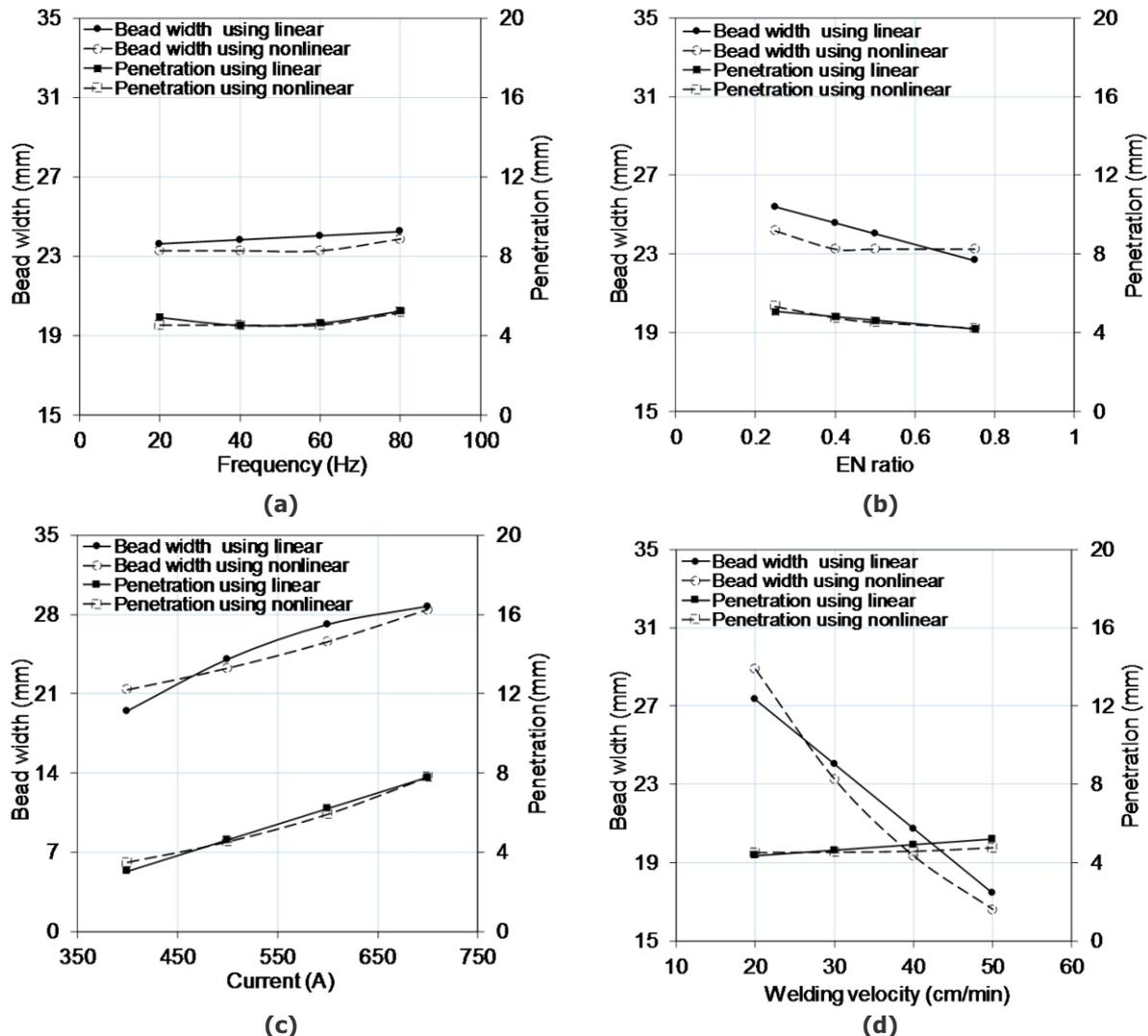
**Fig. 3 :** Effect of (a) frequency at E=0.5, I=500 A and V=30 cm/min (b) EN ratio at F=60 Hz, I=500 A and V=30 cm/min, (c) current at F=60 Hz, E=0.5 and V=30 cm/min (d) welding velocity at F=60 Hz, E=0.5 and I=500 A on bead width and penetration.
