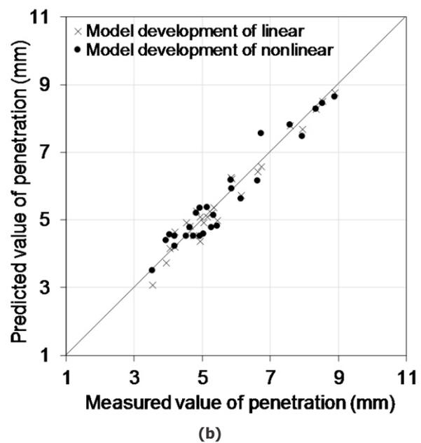
Fig. 2 : Comparison between predicted and measured width and penetration
