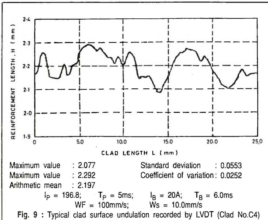
Fig. 9 : Typical clad surface undulation recorded by LVDT (Clad No.C4)
