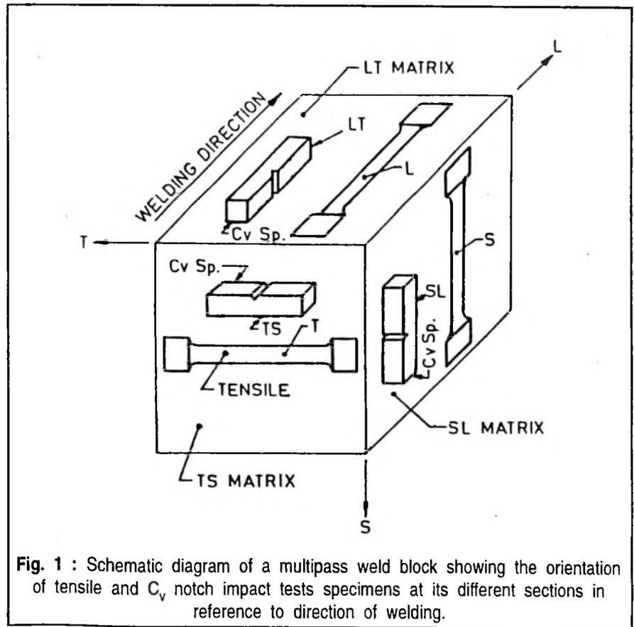
Fig. 1 : Schematic diagram of a multipass weld block showing the orientation of tensile and  $C_v$  notch impact tests specimens at its different sections in reference to direction of welding.
