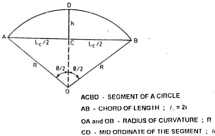
**Fig. 3 :** Schematic diagram of geometric representation of weld bead reinforcement
