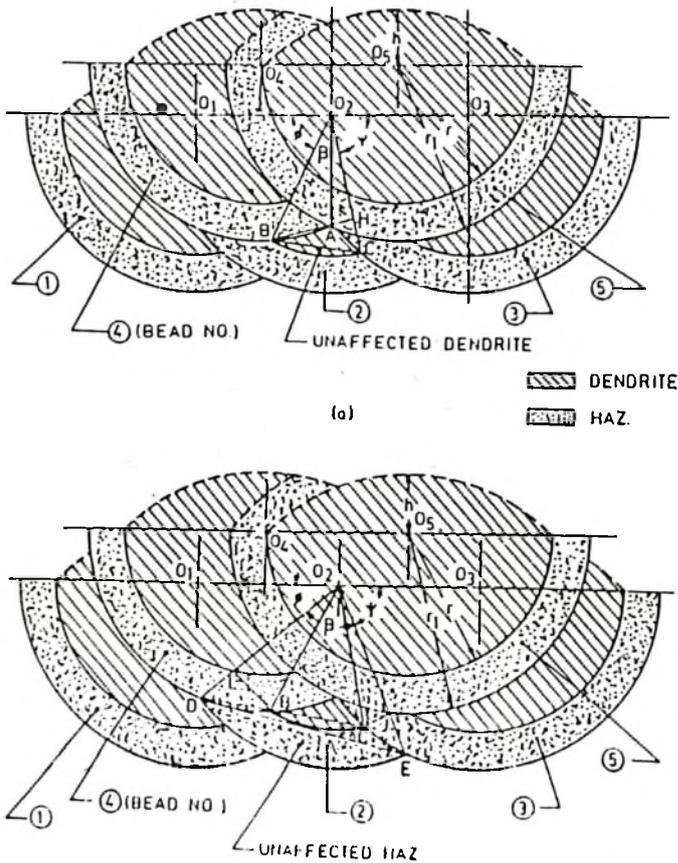
**Fig. 2 :** Geometric model of a multipass weld
