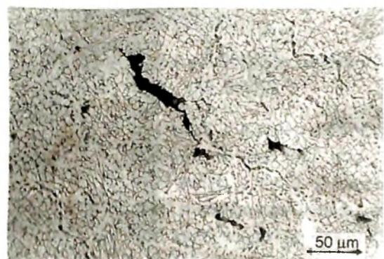
**Fig. 11 :** Microstructures of fusion zone cracking in stabilised stainless steels a) D9 showing cracks in A-mode microstructure and b) type 321 showing fine cracks in FA mode microstructure.
