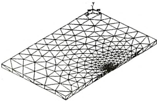
Fig 7 : Type of mesh for 120 mm x 80 mm x 4 mm plate after 18.018 second
