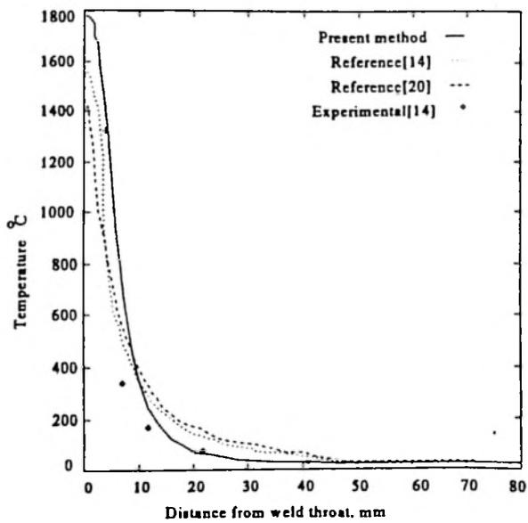
Fig 11 : Transverse temperature distribution at mid section during passing arc
