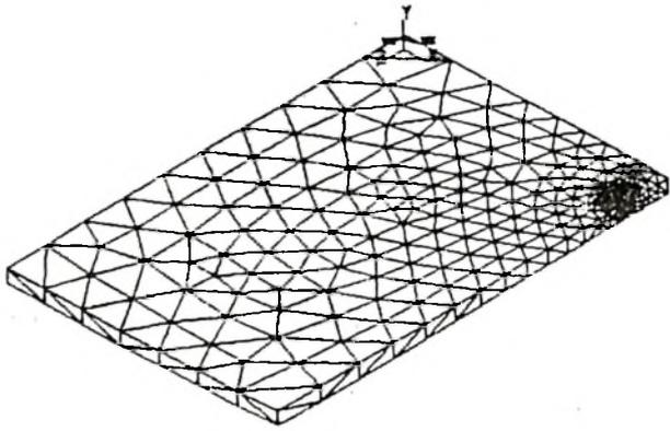
Fig 5 : Type of mesh for 120 mm x 80 mm x 4 mm plate after 3.603 second
