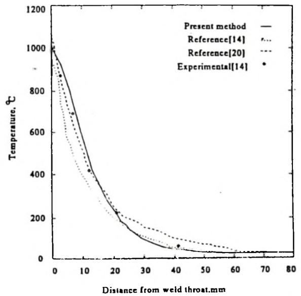
Fig 12 : Transverse temperature distribution at mid section 7.5 s after passing arc
