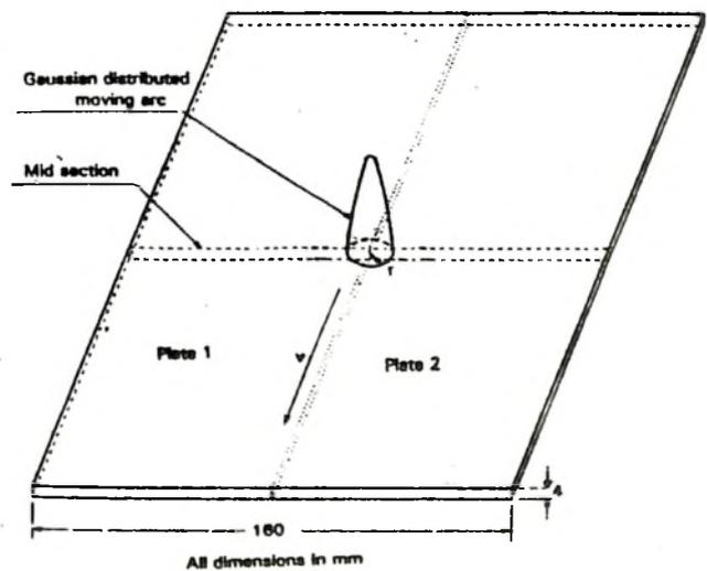
Fig 4 : Arc welding of steel plate
