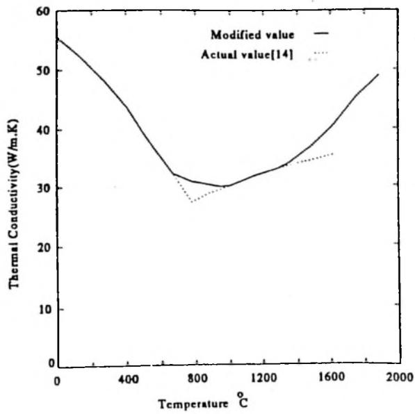
Fig 1 : Thermal Conductivity of mild steel St 37
