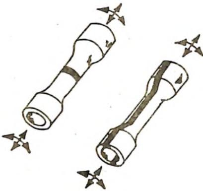
Fig.4: Tubular fatigue specimens for confirmatory tests on fatigue strength reduction factors
