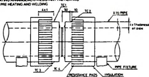
NOTE No of TC Points shall be decided based on pipe thickness and diameter of pipe
