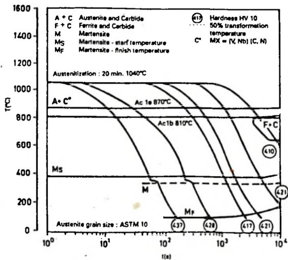
Fig.1 Continuous Cooling Transformation Diagram for the 9% Cr Steel.
