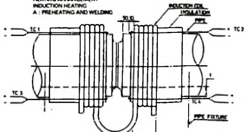
No of turns shall be decided based on the thickness of pipe and diameter of the pipe
