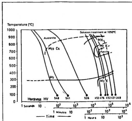
Fig.2 Continuous Cooling Transformation Diagram for X20 Cr Steel Mo V12 1
