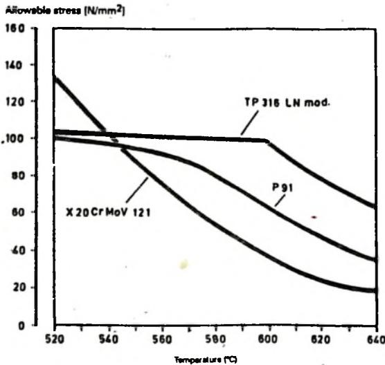
Fig.5: Allowable Stresses for steels TP 316 LN mod., P 91 and X20 Cr MoV 12 1
