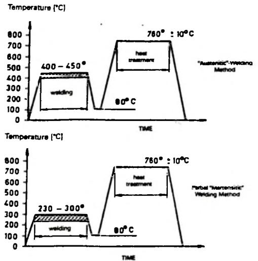
Fig.6: Temperature Regimes for Austenitic and Martensitic welding and PWHT
