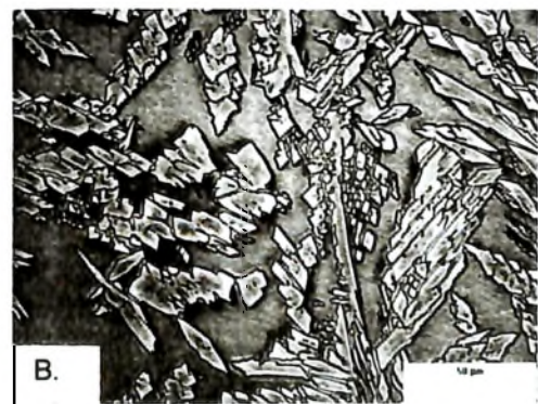
Fig. 5:Micrographic Images of (A) PEAFF-TIG weld metal and (B) Traditional GTAW weld metal
