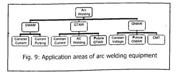
AWE feeds energy to arc welding process. It should be electrically efficient and ensure process compatibility i.e. it should meet productivity with requisite weld quality. High productivity directly enhances  $E^2$ . Table IV lists down certain comparison of regularly used rectifier based welding modes.
