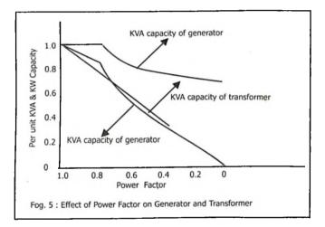
on incurred loss. Prolonged overheating reduces their life. Poor pf with large harmonics reduces the power delivery capacity of these equipments resulting under utilization. Additional facility calls for large infrastructure cost, energy waste etc. It is difficult and complex activity to implement  $E^2$  in large installations.
