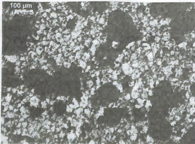
**Fig. 7 : Optical micrograph of friction stir weld after corrosion**
