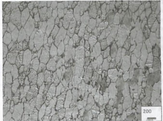
**Fig. 4 : Microstructure of FS weld**
