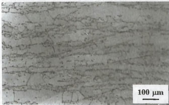
**Fig. 2 : Microstructure of Base metal**
