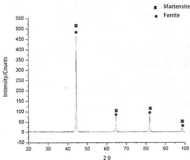
**Fig.8 : XRD results of martensite in the stir zone of friction stir weld**
