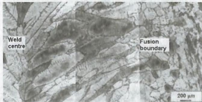
**Fig. 3 : Microstructure of GTA weld**
