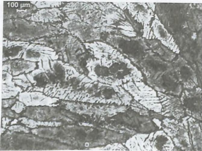
**Fig. 6 : Optical micrographs of GTA weld after corrosion**
