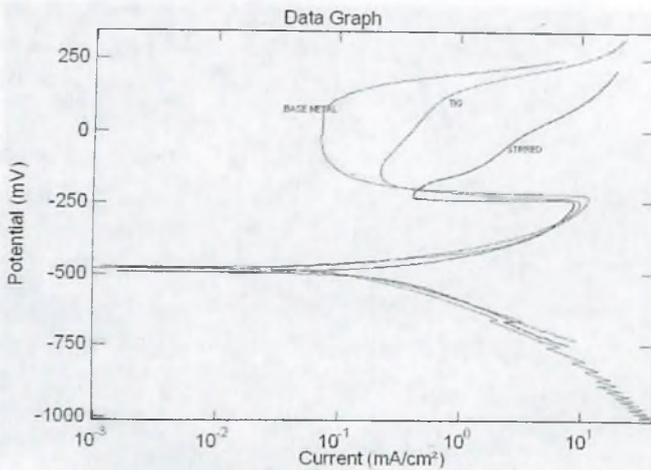
**Fig. 5 : Potentio-dynamic polarization curves of GTA and FS welds**
