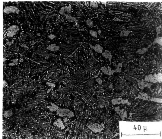
Fig. 3 : Light micrograph of the base material
