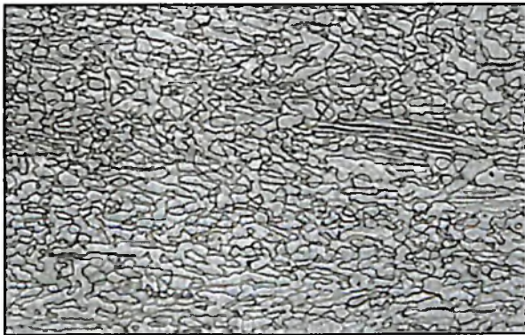
Micro report 6: Coarse grained elongated structure produced in Ti-6 Al 4V alloy, by light forging reduction, annealed, X100.
