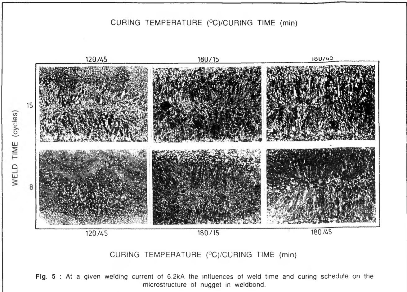
shown in **Fig.6**. The micrographs presented in **Figs. 5** and **6** show that the increase in energy input with the increase of welding current or weld time enhances the coarsening and recrystallization of microstructure of the weld nugget. It is also observed that the increase in curing temperature and time does not have any significant influence on the microstructure of the weld nugget.
