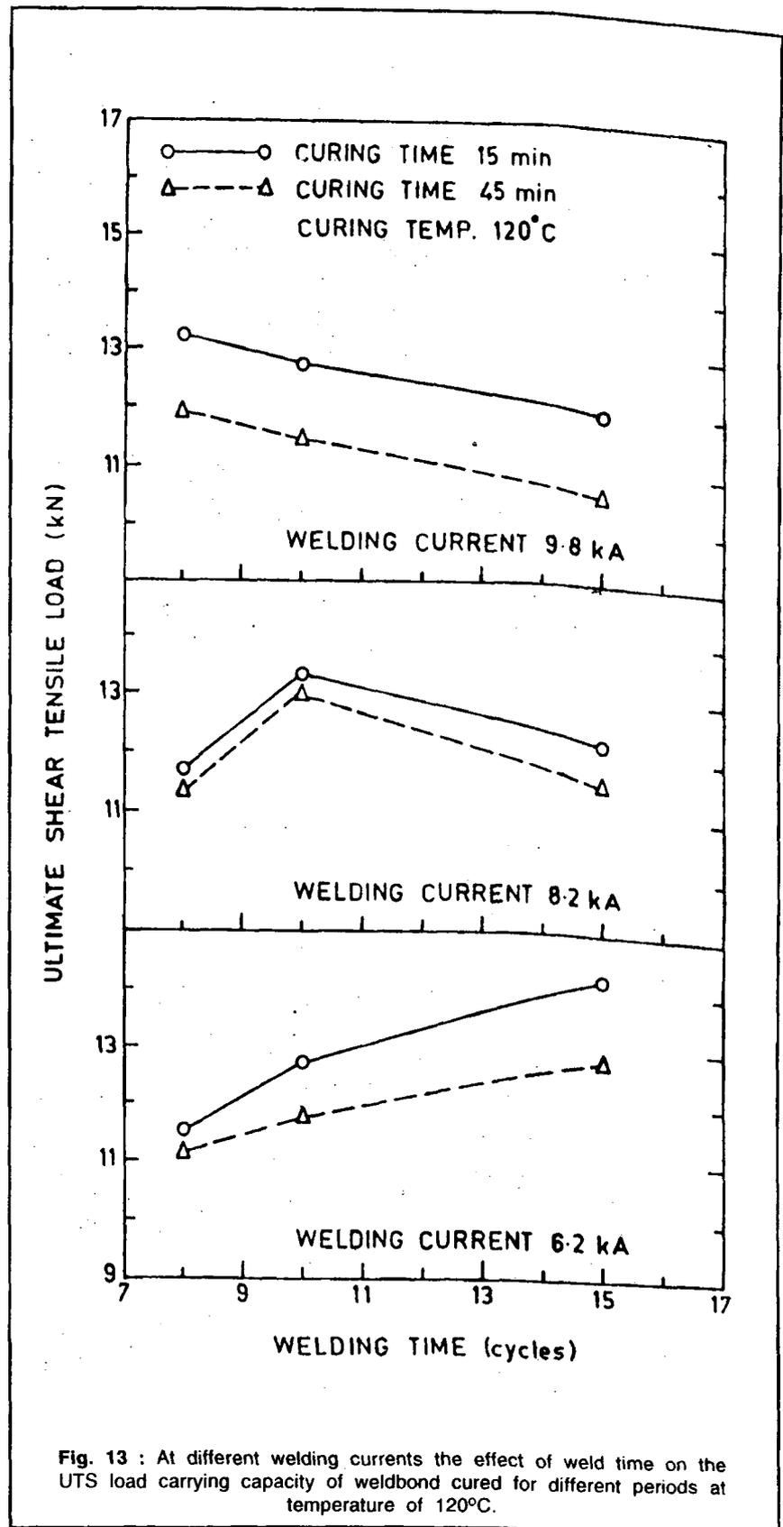
Fig. 13 : At different welding currents the effect of weld time on the UTS load carrying capacity of weldbond cured for different periods at temperature of 120°C.
