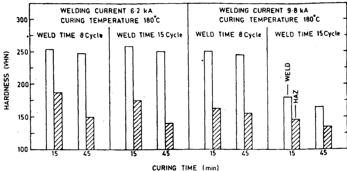
Fig. 9 : At different welding currents and times the influence of curing time on the hardness of weld and HAZ of weldbond cured at temperature of 180°C.
