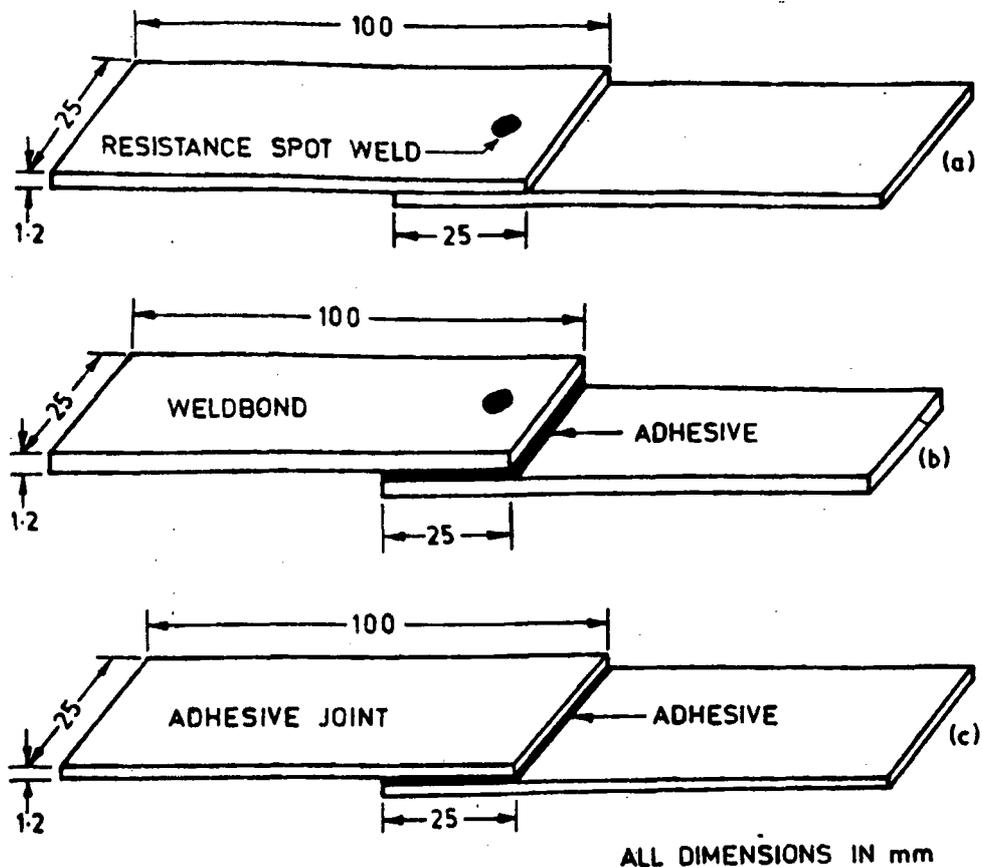
Fig. 1 : Schematic diagram of the shear-tensile test specimen;
