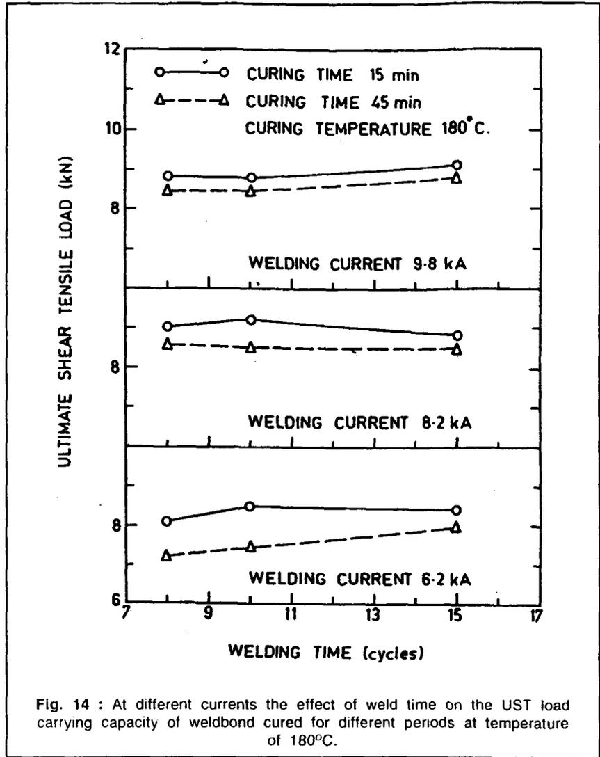
Fig. 14 : At different currents the effect of weld time on the UST load carrying capacity of weldbond cured for different periods at temperature of 180°C.
