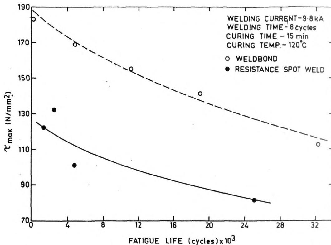
Fig. 15 : Comparison of fatigue life of the resistance spot weld and weldbond prepared at a given welding current and weld time.
