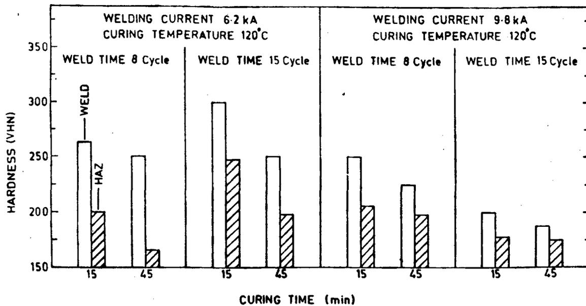
Fig. 8 : At different welding currents and times the influence of curing time on the hardness of weld and HAZ of weldbond cured at temperature of 120°C.
