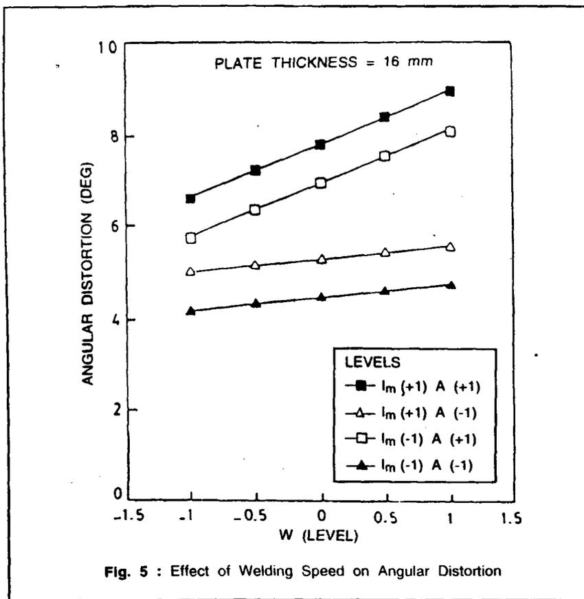
Fig. 5 : Effect of Welding Speed on Angular Distortion
