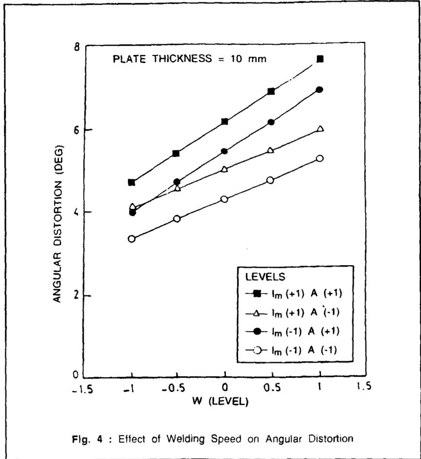
Fig. 4 : Effect of Welding Speed on Angular Distortion
