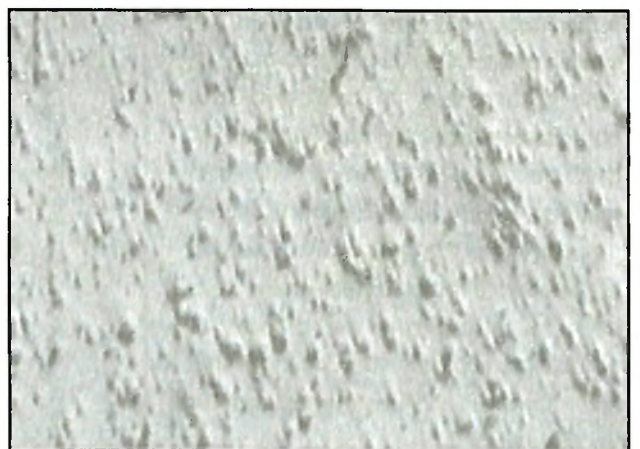
Fig-11 : Microstructure at the non-welded zone of 50 Magnification for 22 kJ/mm Heat Input
