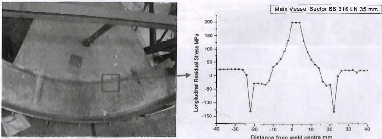
**Fig. 16 : (a) Sector of the main vessel with the location of the weld marked in box. (b) Variation in longitudinal residual stress in 35 mm thick single "V" AISI type 304 stainless steel weld region as determined by the LCR wave transit time measurements.**
