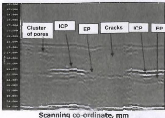
Fig. 10 : TOFD image for different defects in weld pad
