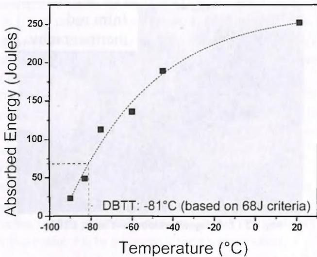
**Fig. 26 : Variation of Impact toughness of the weld metal produced by RAFM filler wire**
