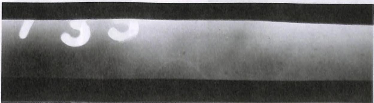
**Fig. 18 :** Microfocal radiography image of a typical TTS weld joint with micro-porosities.
