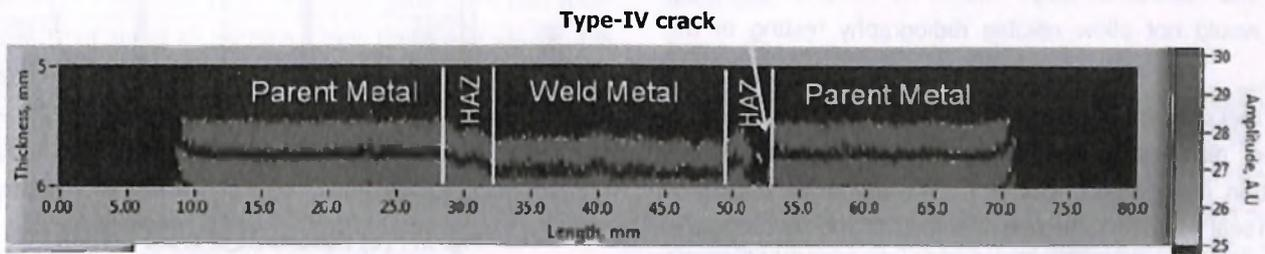
**Fig. 15 : Ultrasonic b-scan image of the back wall echo across a ferritic steel weld subjected to creep at 923 K / 50 MPa for 1992 h.**
