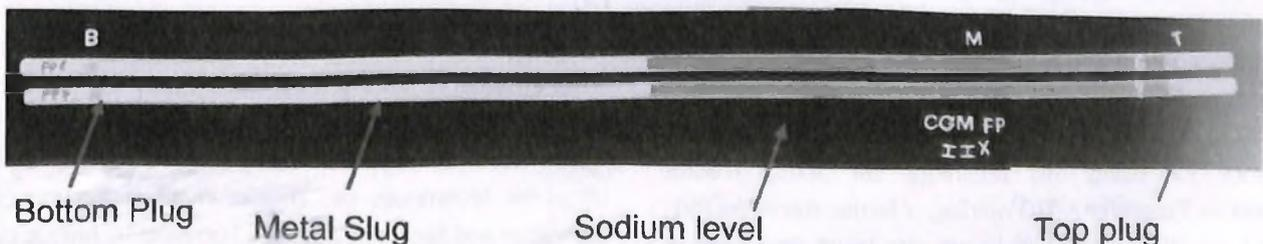
**Fig. 6 : Radiography image of metallic fuel pins containing fuel and sodium made using modified 9Cr-1 Mo steel clad tube and end plug**
