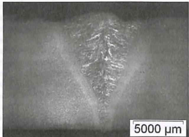
**Fig. 28 : Macrostructure of laser hybrid weld produced using 12 mm thick RAFM steel**
