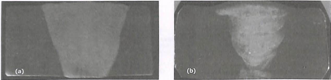
Fig. 7 : Macrograph of 10 mm thick austenitic stainless steel (a) A-TIG and (b) conventional TIG
