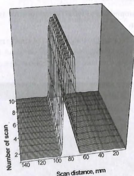
**Fig : 19 (b) High temperature ECT based image of the weldment**
