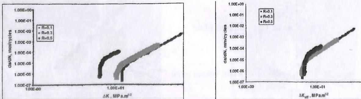
Fig. 22 : Variation in FCG behaviour with  $\Delta P_{eff}$  estimated using a)conventional method and b) using acoustic emission data collected during FCG test.
