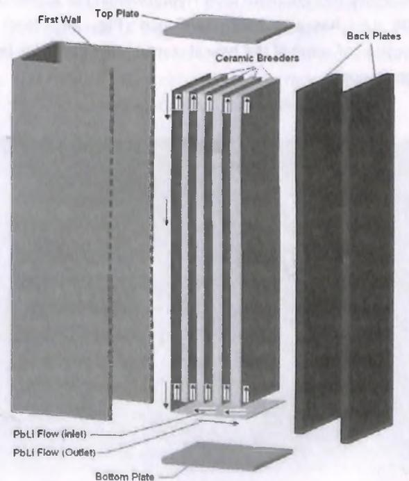
Fig. 25 : Schematic of important components of Indian TBM
