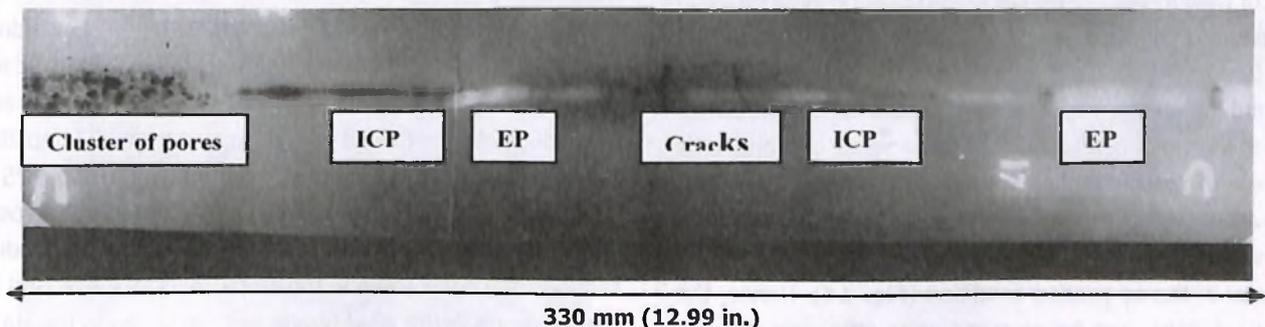
Fig. 9 : Radiograph showing planar location of different defects in the weld pad ICP (Incomplete penetration), EP (-Excess Penetration)
