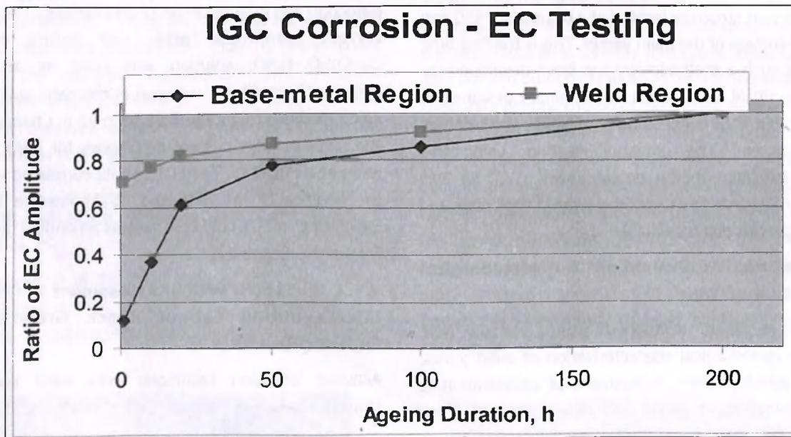
Fig. 21 : Ratio of EC amplitudes of aged exposed (Cu-CuSO<sub>4</sub>-H<sub>2</sub>SO<sub>4</sub> – Strauss Test) to unexposed Base metal prone to sensitization, weld metal is resistant to sensitization
