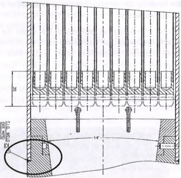
**Fig. 17: (a) Schematic of cross section of hexagonal wrapper tube with fuel pins showing the seal weld location**
