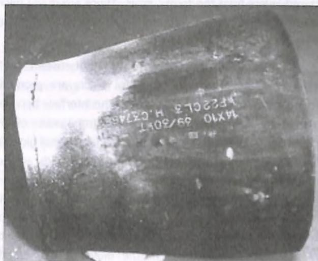
**Fig. 29 : Photograph of the failed reducer**
