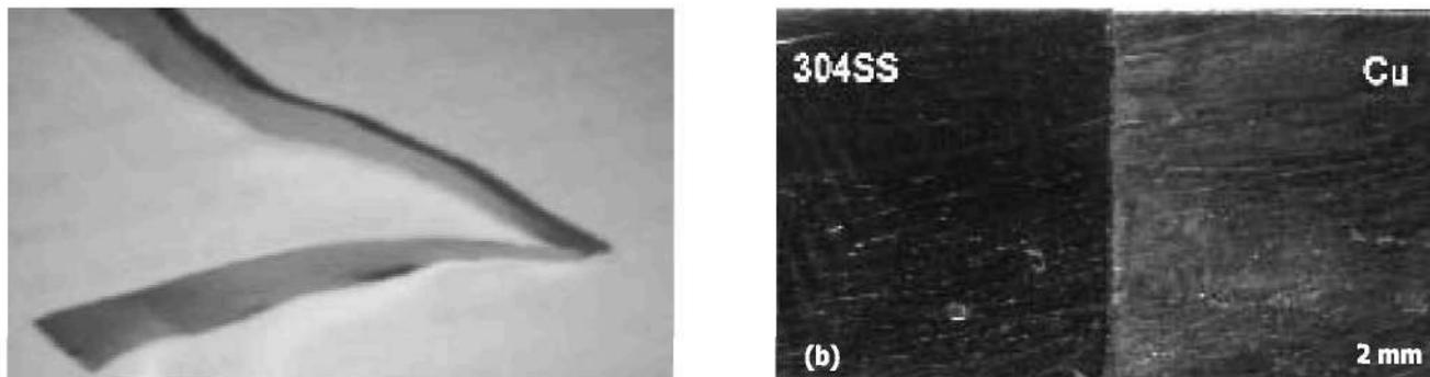
**Fig. 2 : Developed brazing foil shows (a) 180° folding and (b) successful joint between 304SS and Cu**
