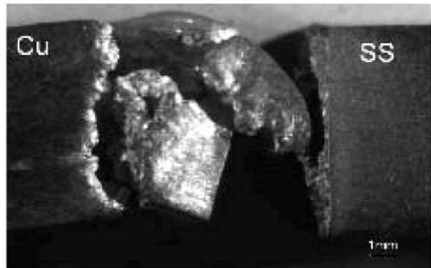
Fig. 5 : Photographs of fracture surface of 304SS-Cu joint brazed by C50 alloy (a) at 920°C, (b) at 980°C
