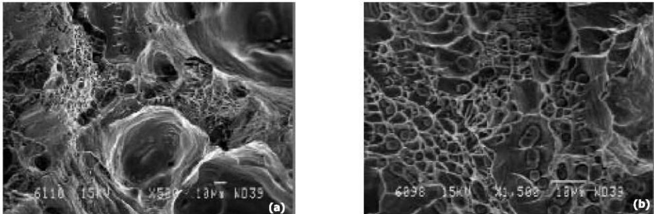
Fig. 6 : Fractographs of the butt joint at (a) SS substrate, (b) Cu substrate
