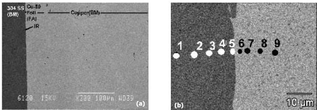
**Fig. 3 : SEM-BSE image of 304 SS-Cu brazed joint showing (a) Porosities free joint area (b) EDS elemental analysis at different points**
