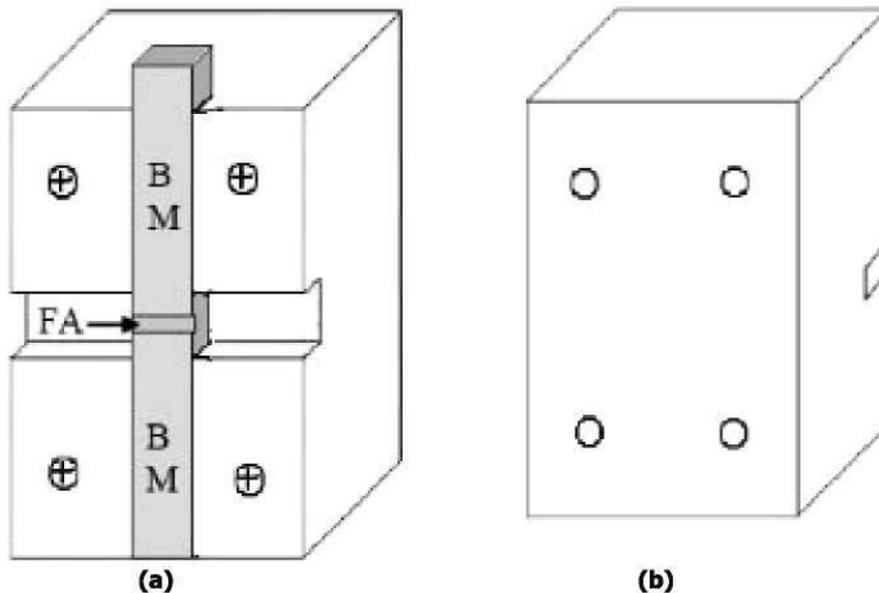
**Fig. 1 : Schematic diagram of brazement assembly showing (a) Bottom part and (b) Top part of brazing jigs (BM: Base metal and FA: Filler alloy)**
