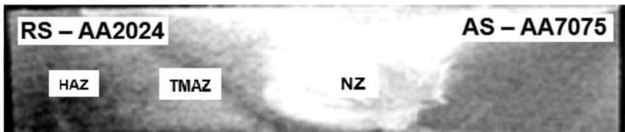
Fig.2 : Typical cross section of the weld (600rpm, 30mm/min, 2.5kN, Taper cyl. threaded tool)
