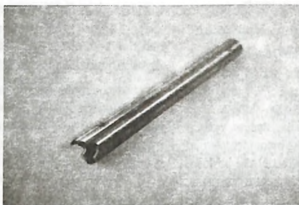
Fig. 5 : Special tool designed and used for removing MgO powder
