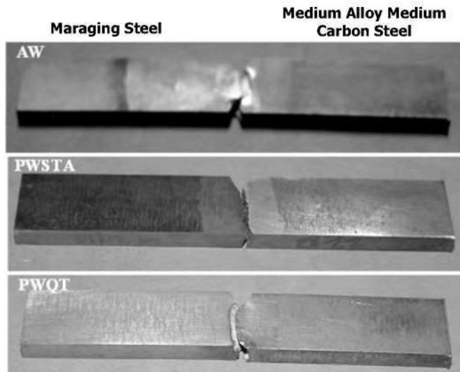
**Fig.9: Impact test samples of dissimilar metal gas tungsten arc weldment of maraging steel and medium alloy medium carbon steel with maraging steel filler in various heat treated conditions**
