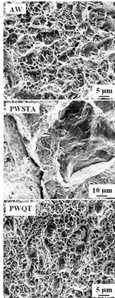
**Fig.12 : Fractographs of impact samples of dissimilar metal gas tungsten arc weldment of maraging steel and medium alloy medium carbon steel with medium alloy medium carbon steel filler in various heat treated conditions**
