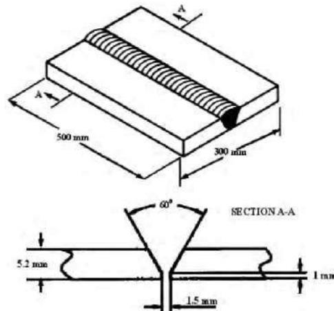
Fig. 1 : Weld coupon design and test place assembly
