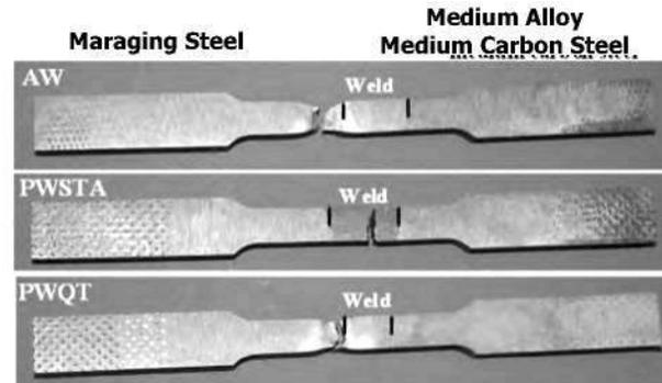
**Fig.5 : Fracture location of tensile samples of dissimilar metal gas tungsten arc weldment of maraging steel and medium alloy medium carbon steel with maraging steel filler in various heat treated conditions**
