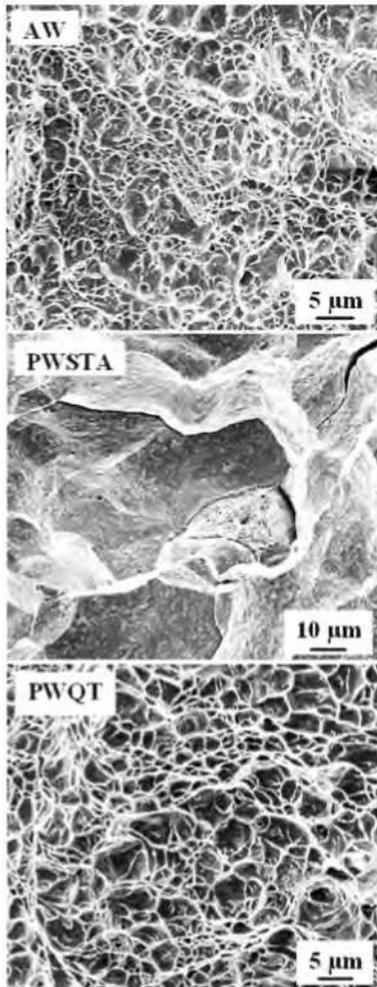
**Fig.10: Fractographs of impact samples of dissimilar metal gas tungsten arc weldment of maraging steel and medium alloy medium carbon steel with maraging steel filler in various heat treated conditions**
