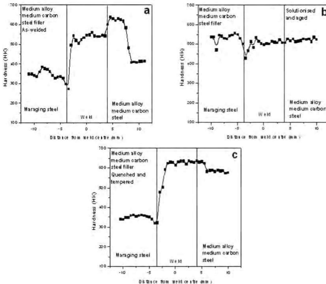
**Fig.4 : Hardness traverse across the dissimilar metal gas tungsten arc weldment of maraging steel and medium alloy medium carbon steel with medium alloy medium carbon steel filler in various heat treated conditions (a) As-welded (b) Solutionised and Aged (c) Quenched and tempered**
