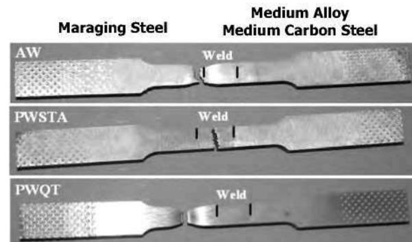
**Fig.7 :** Fracture location of tensile samples of dissimilar metal gas tungsten arc weldment of maraging steel and medium alloy medium carbon steel with medium alloy medium carbon steel filler in various heat treated conditions
