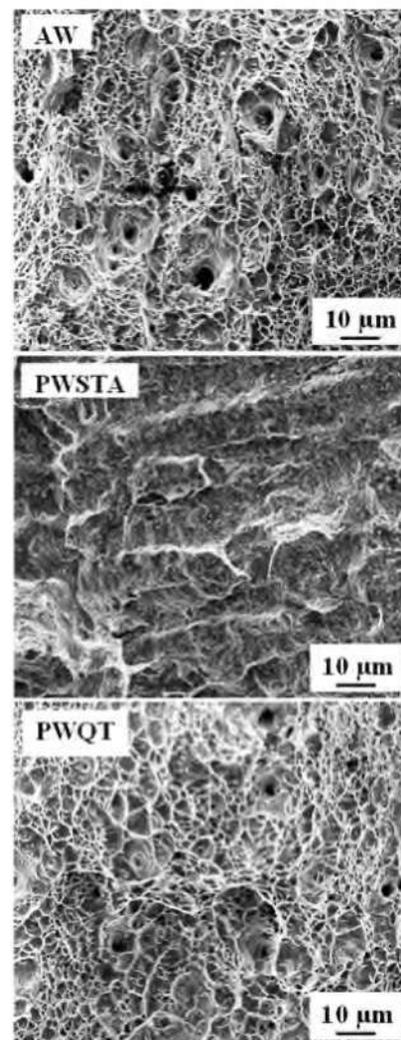
**Fig.8 :** Fractographs of tensile samples of dissimilar metal gas tungsten arc weldment of maraging steel and medium alloy medium carbon steel with medium alloy medium carbon steel filler in various heat treated conditions
