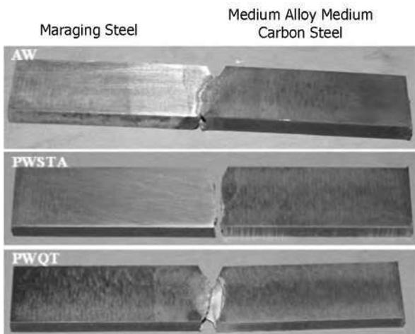
**Fig.11 : Impact test samples of dissimilar metal gas tungsten arc weldment of maraging steel and medium alloy medium carbon steel with medium alloy medium carbon steel filler in various heat treated conditions**
