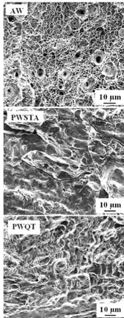
**Fig.6 : Fractographs of tensile samples of dissimilar metal gas tungsten arc weldment of maraging steel and medium alloy medium carbon steel with maraging steel filler in various heat treated conditions**
