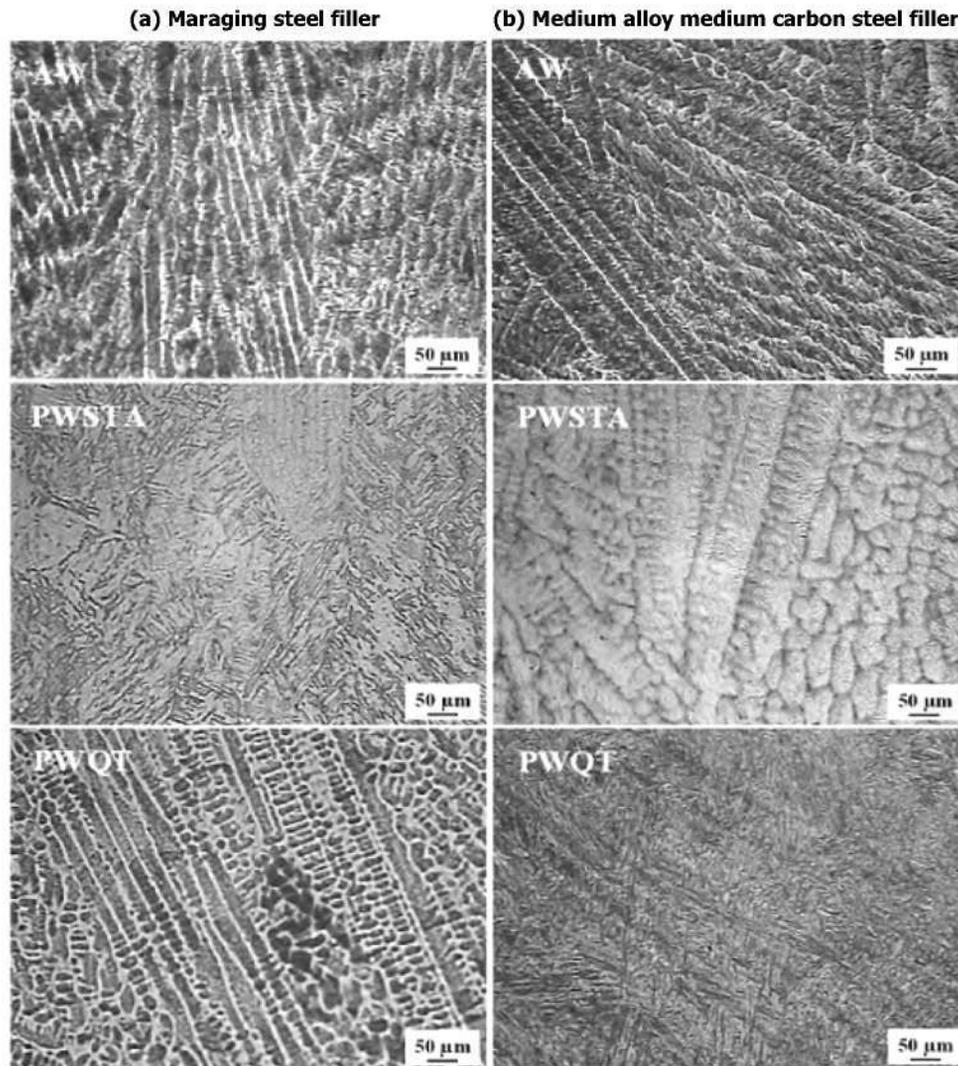
**Fig.2 : Optical microstructure of weld centre of dissimilar metal gas tungsten arc weldment of maraging steel and medium alloy medium carbon steel with (a) maraging steel filler (b) medium alloy medium carbon steel filler, in various post-weld heat treated conditions**
